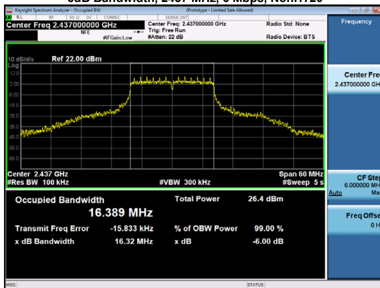
6dB Bandwidth, 2437 MHz, 6 Mbps, NonHT20
