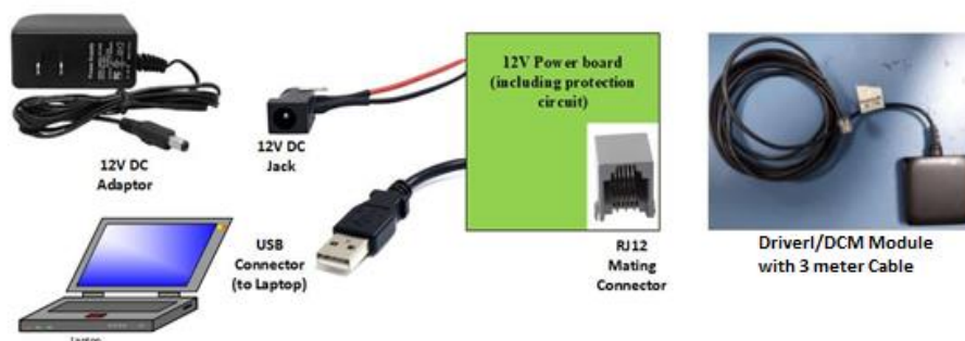
Figure 10: DriverI/DCM module complete setup with Power Board
