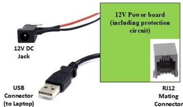
Figure 9: Power Board with DriverI/DCM Setup
