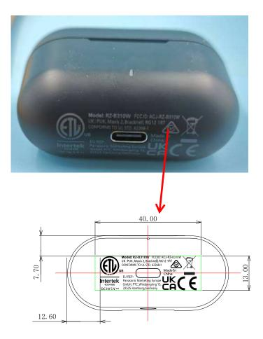
The marking information is located at the bottom of charging case
