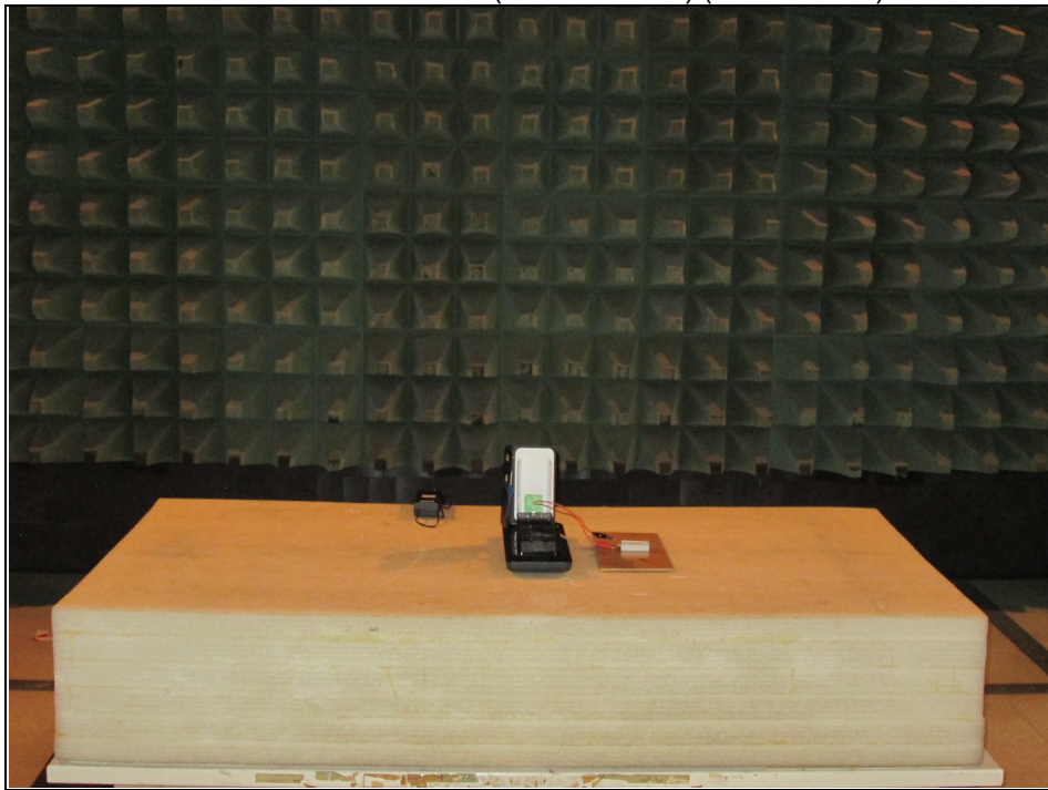
Radiated Emission Test (above 30MHz) (Test Mode A)
