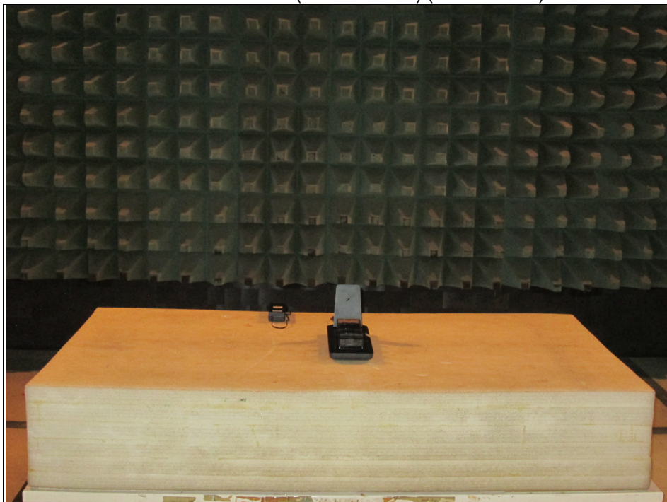
Radiated Emission (9kHz~30MHz) (Test Mode B)
