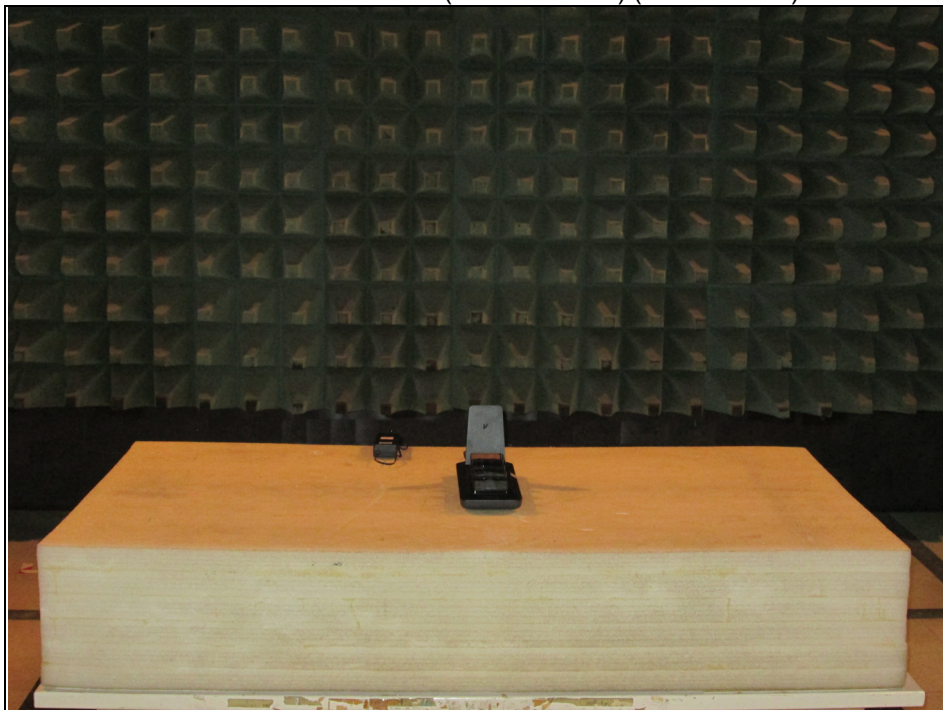
Radiated Emission Test (above 30MHz) (Test Mode B)
