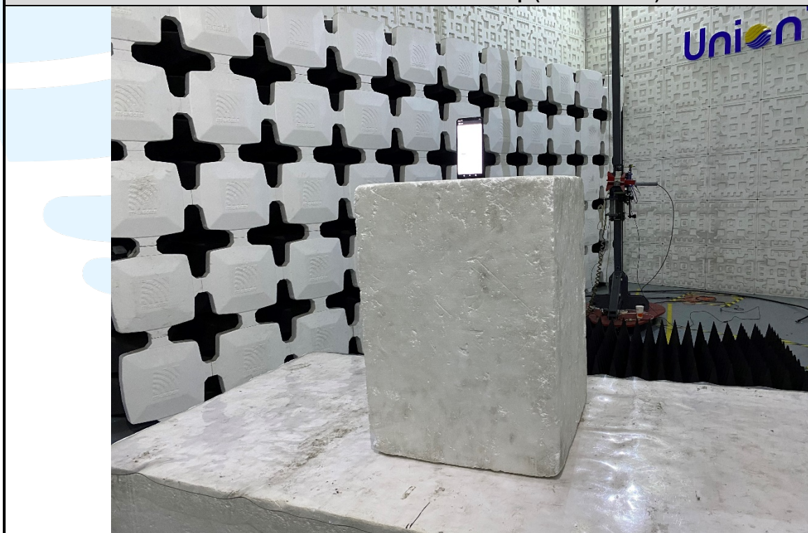
Radiated emission Test Setup (Above 1 GHz)
