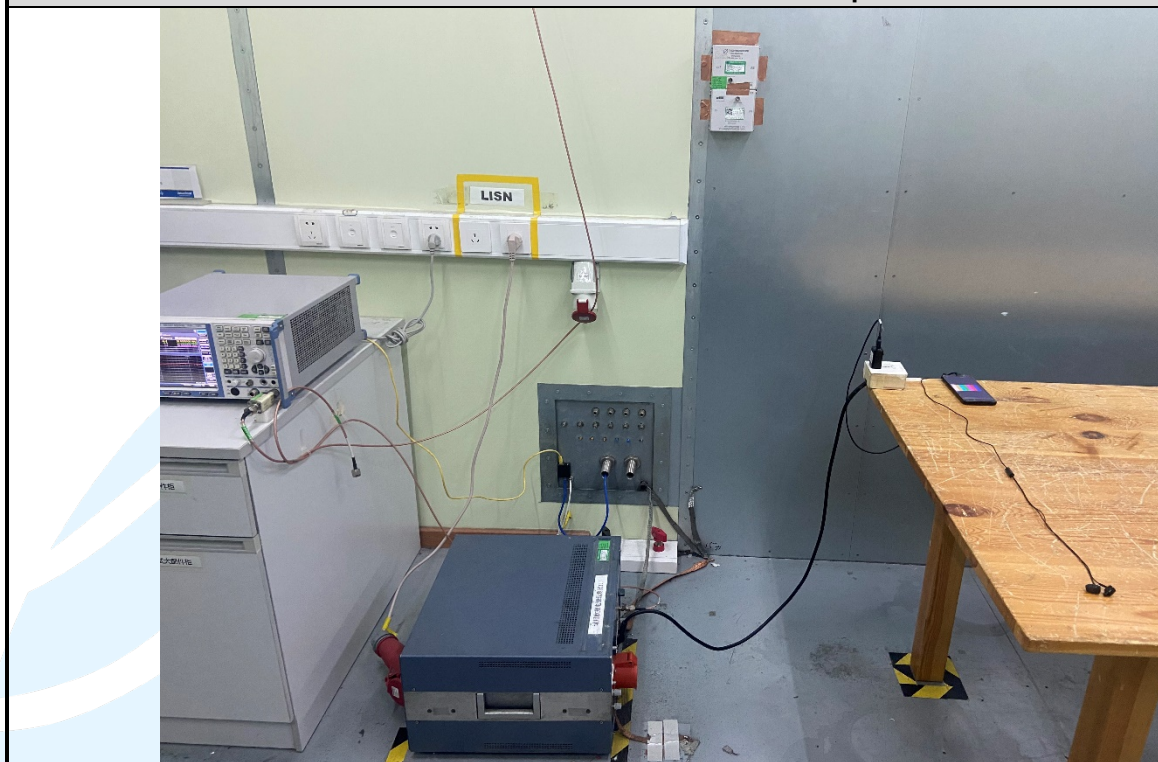
Conducted Emission Test Setup
