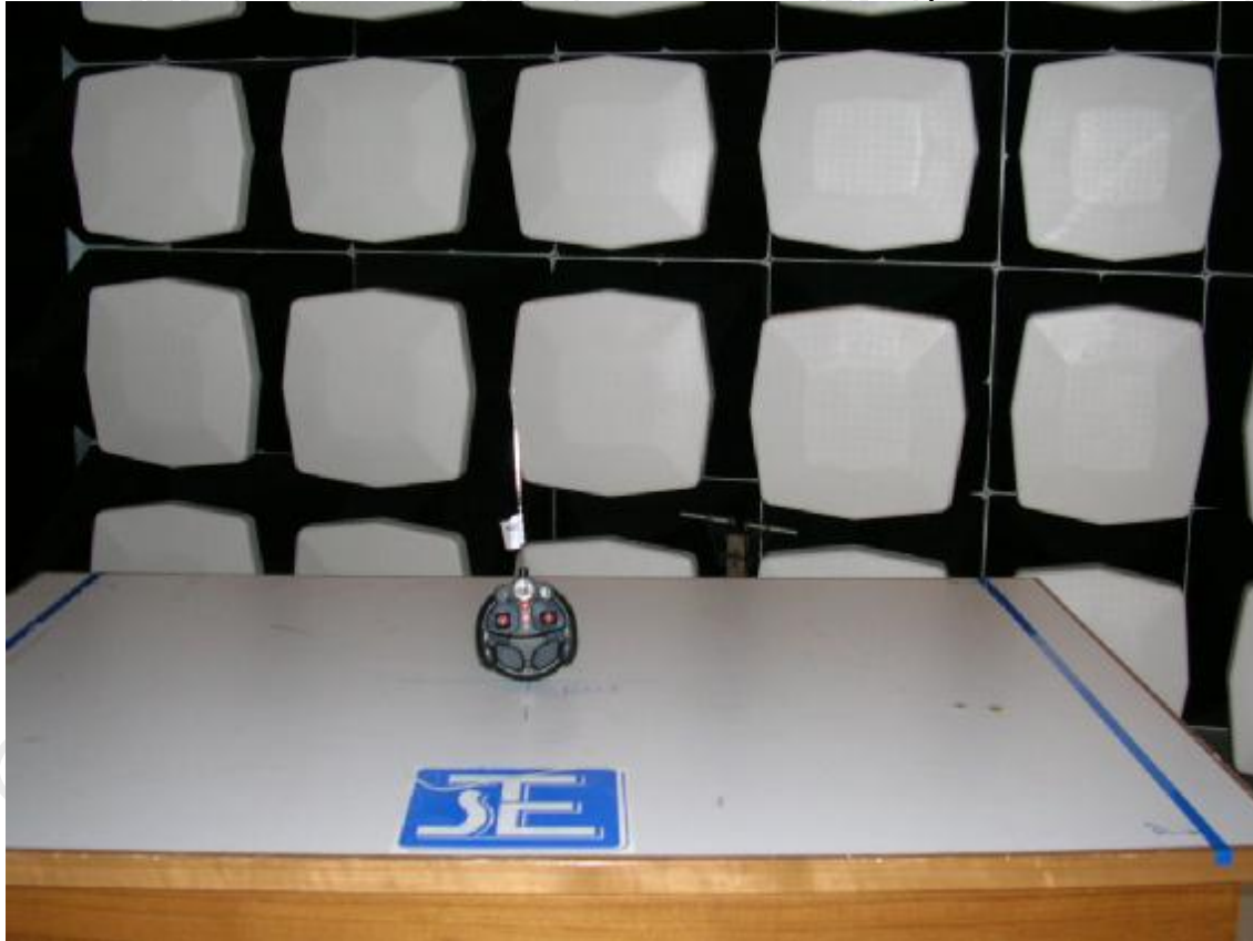
Measurement of Radiated Emission Test Set Up
