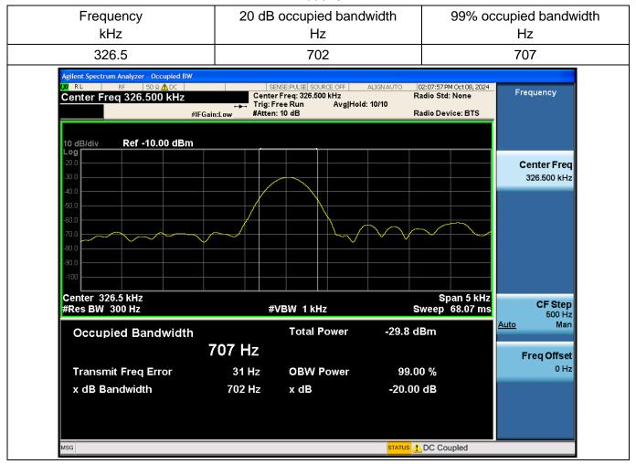
**Note:** Because the measured signal is CW-like, adjusting the RBW per C63.10 would not be practical since measurement bandwidth will always follow the RBW. The RBW is set to 300 Hz to perform the
