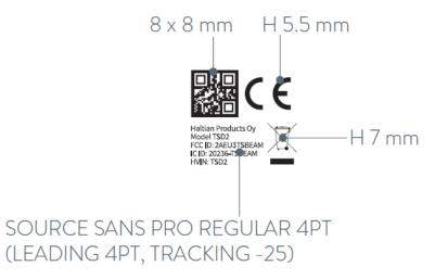
The markings are done by laser to the device cover
