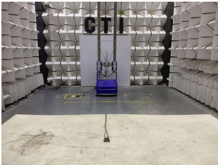
Radiated spurious emission Test Setup-1(Below 1GHz)
