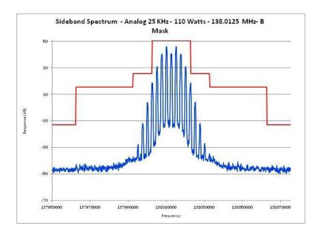
E1-5.9 Occupied Bandwidth, Analog, 25 kHz Channels, 138.0125 MHz PL
