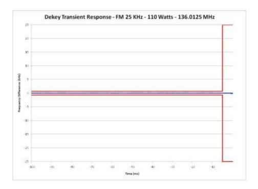
E1-9.6 Frequency Transient Behavior, 25 kHz Channel De-Key, 138.0125 MHz
