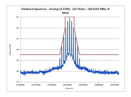
E1-5.21 Occupied Bandwidth, Analog, 12.5 kHz Channels, 138.0125 MHz PL
