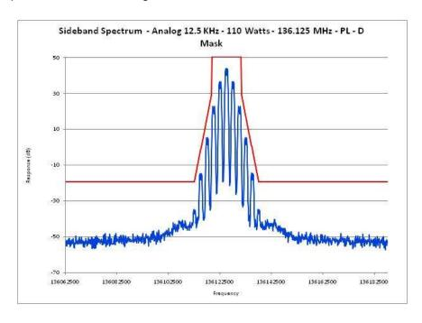
E1-5.19 Occupied Bandwidth, Analog, 12.5 kHz Channels, 136.0125 MHz DPL
