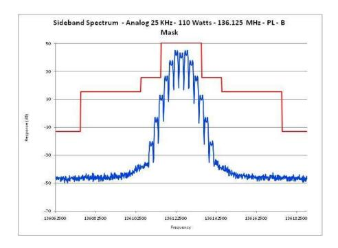
E1-5.7 Occupied Bandwidth, Analog, 25 kHz Channels, 136.0125 MHz DPL
