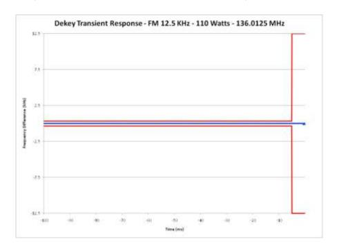
E1-9.14 Frequency Transient Behavior, 12.5 kHz Channel De-Key, 138.0125 MHz
