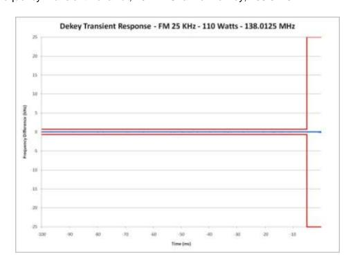
E1-9.7 Frequency Transient Behavior, 25 kHz Channel De-Key, 155.0125 MHz
