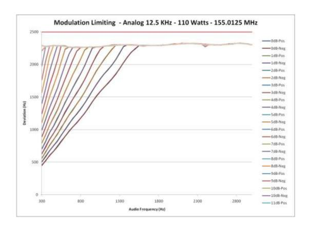
E1-11.8 Audio Modulation Limiting – Modulation Characteristics, 12.5 kHz Channels – 173.9875 MHz
