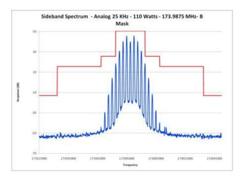
E1-5.15 Occupied Bandwidth, Analog, 25 kHz Channels, 173.9875 MHz PL
