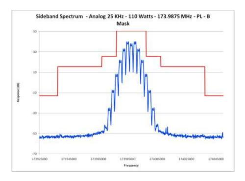
E1-5.16 Occupied Bandwidth, Analog, 25 kHz Channels, 173.9875 MHz DPL
