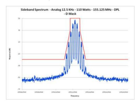
E1-5.26 Occupied Bandwidth, Analog, 12.5 kHz Channels, 173.9875 MHz
