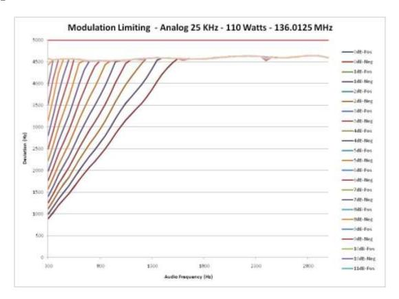
E1-11.2 Audio Modulation Limiting – Modulation Characteristics, 25 kHz Channels – 138.0125 MHz
