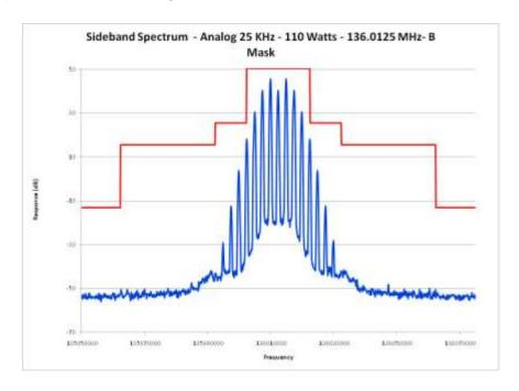
E1-5.6 Occupied Bandwidth, Analog, 25 kHz Channels, 136.0125 MHz PL
