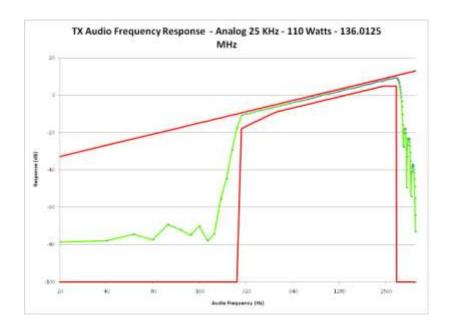
E1-10.2 Audio Frequency Response – Modulation Characteristics, 25 kHz Channels – 138.0125 MHz
