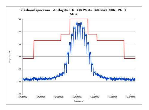
E1-5.10 Occupied Bandwidth, Analog, 25 kHz Channels, 138.0125 MHz DPL
