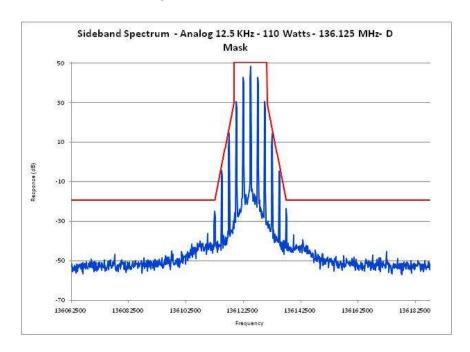
E1-5.18 Occupied Bandwidth, Analog, 12.5 kHz Channels, 136.0125 MHz PL
