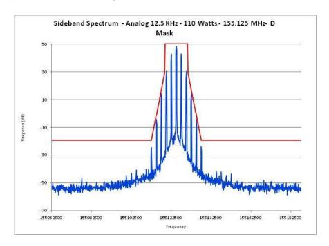
E1-5.24 Occupied Bandwidth, Analog, 12.5 kHz Channels, 155.0125 MHz PL
