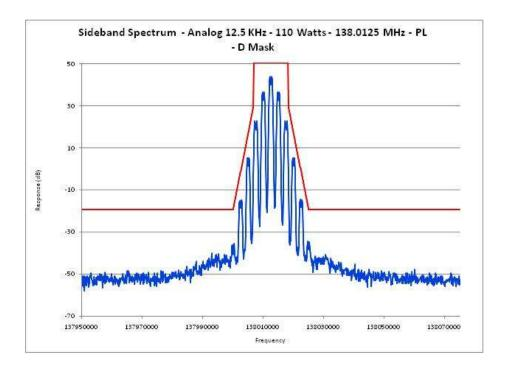
E1-5.22 Occupied Bandwidth, Analog, 12.5 kHz Channels, 138.0125 MHz DPL
