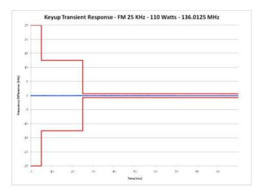
E1-9.2 Frequency Transient Behavior, 25 kHz Channel Key-Up, 138.0125MHz
