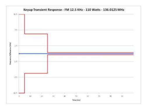
E1-9.10 Frequency Transient Behavior, 12.5 kHz Channel Key-Up, 138.0125 MHz
