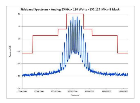
E1-5.12 Occupied Bandwidth, Analog, 25 kHz Channels, 155.0125 MHz PL
