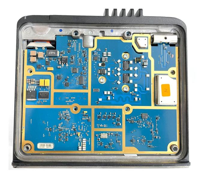
Exhibit 9H: Radio Assembly - Controller Board (Bottom View)
