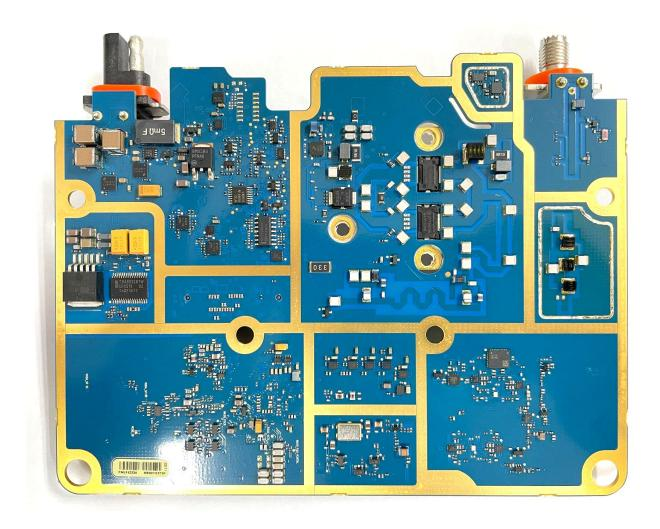
Exhibit 9C: RF board with Shields (Bottom)
