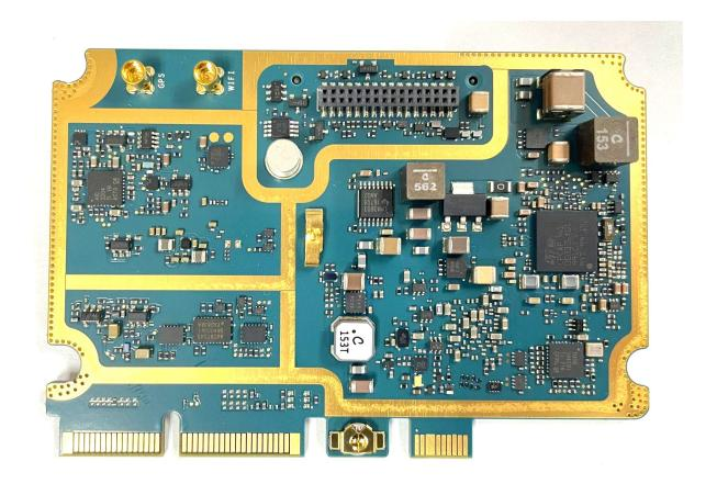
Exhibit 9G: Radio Assembly – RF Board (Top View)
