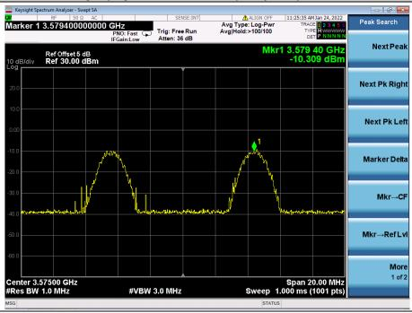
EIRP PSD=-10.309+1=-9.039dBm/MHz, Antenna gain is 1dBi.
