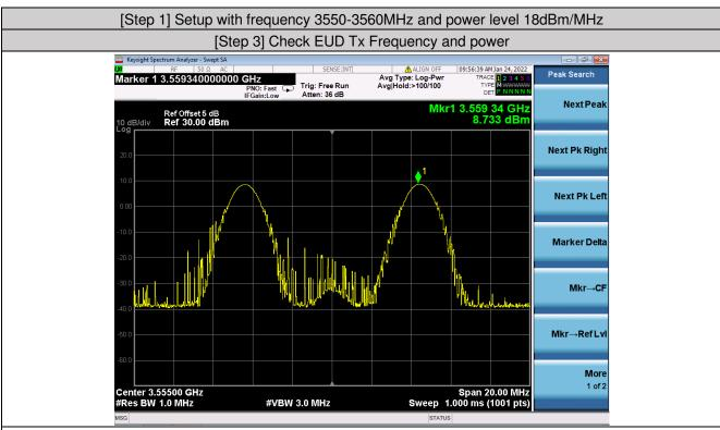
EIRP PSD=8.733+1=9.733dBm/MHz, Antenna gain is 1dBi.
