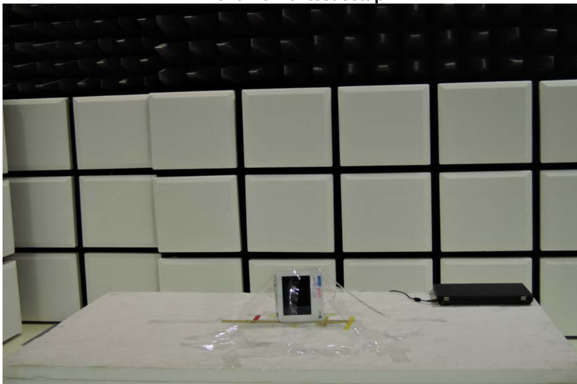
AC Power-line Conducted Emission Set up Photo
