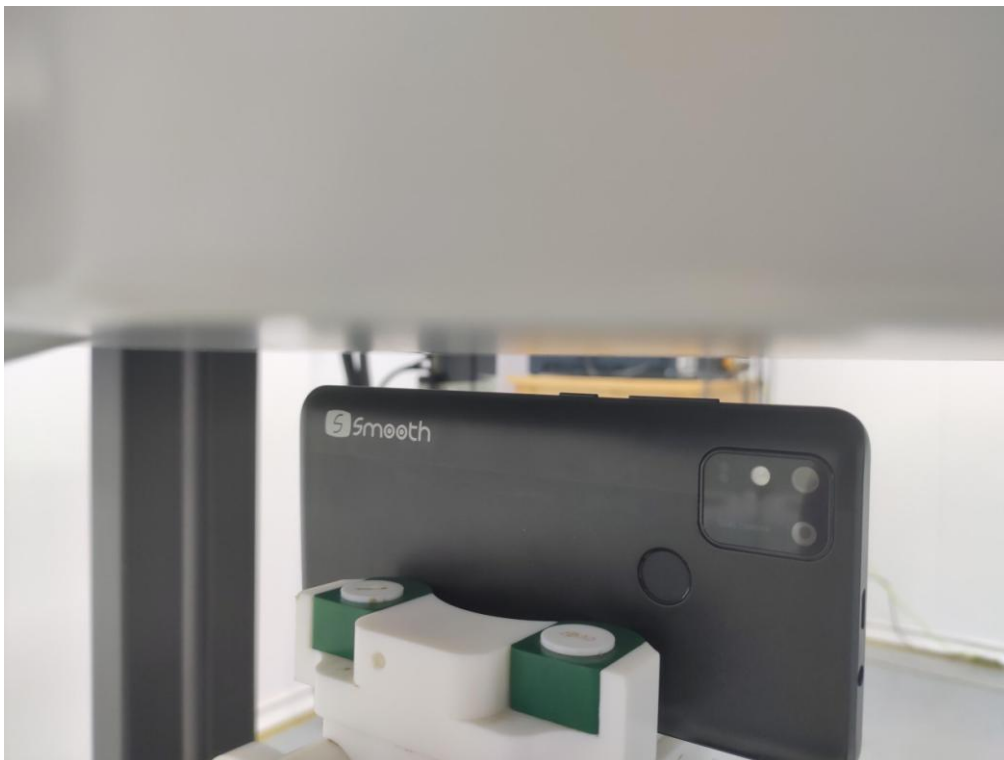
10mm body-worn Right Side Setup Photo (hotspot)
