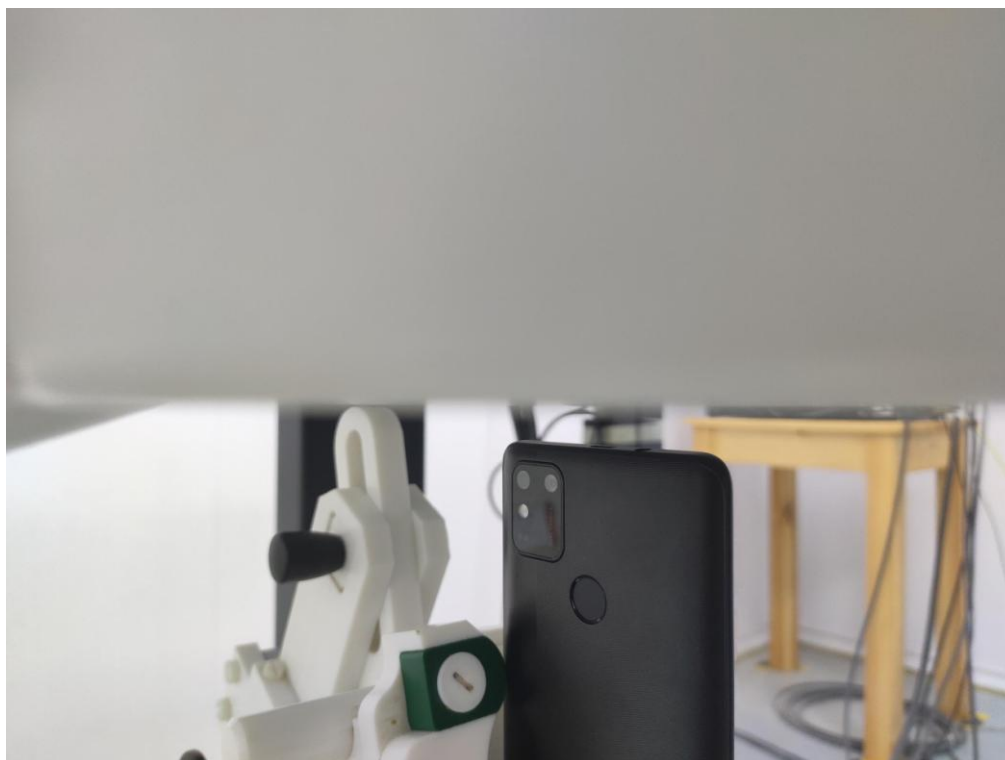
10mm body-worn Top Side Setup Photo (hotspot)
