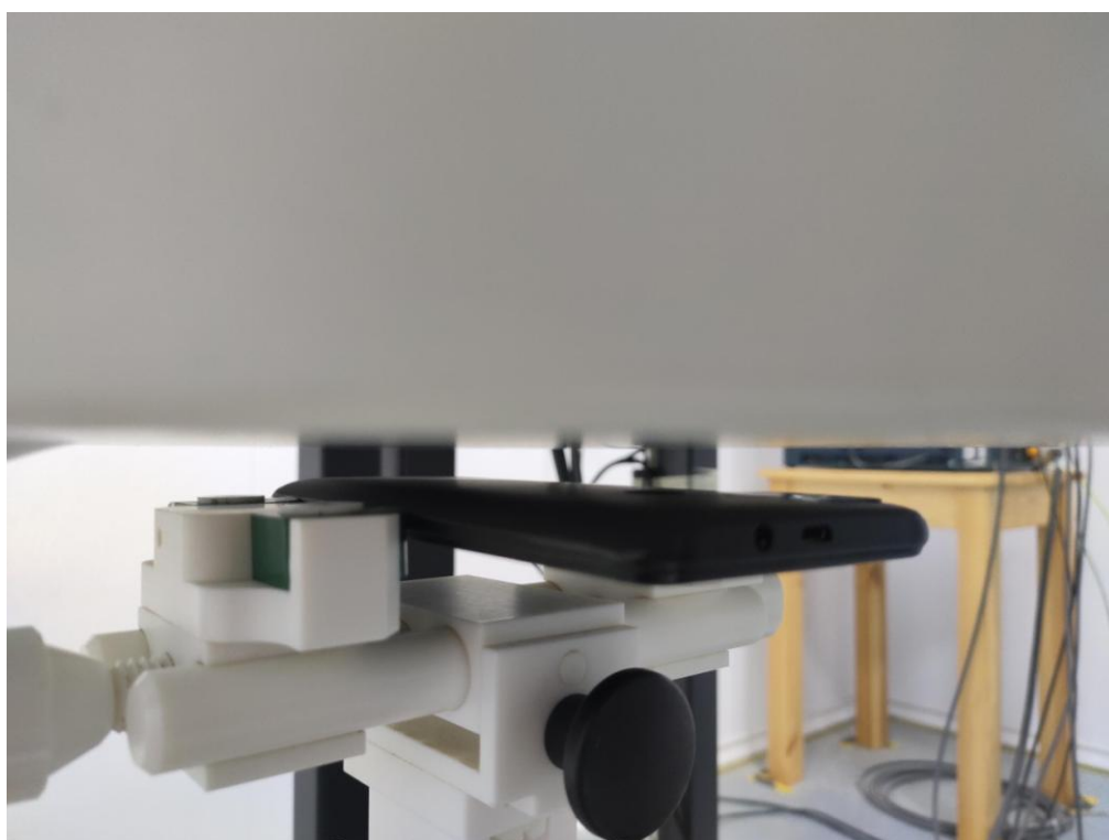
10mm body-worn Back Side Setup Photo (hotspot)
