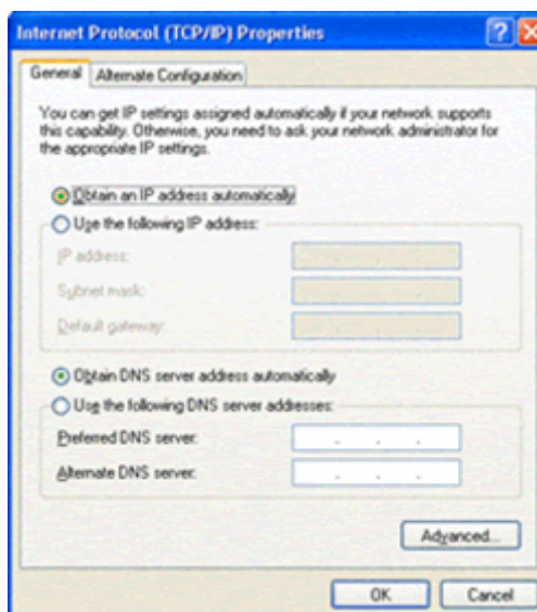
FIGURE 5. Internet Protocol (TCP/IP) Properties
