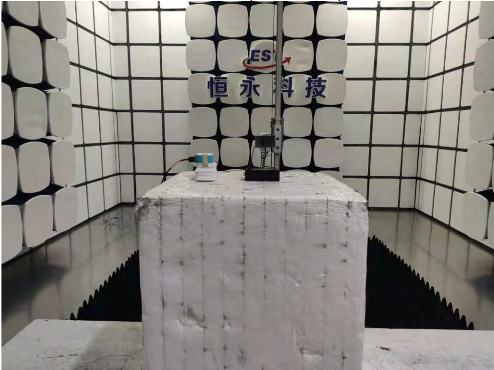
Radiated Test (Above 1GHz)
