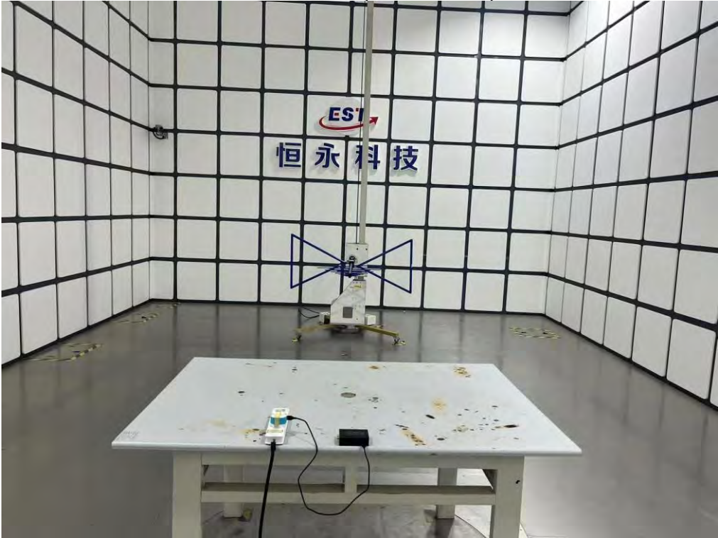
Radiated Test (Below 1GHz)
