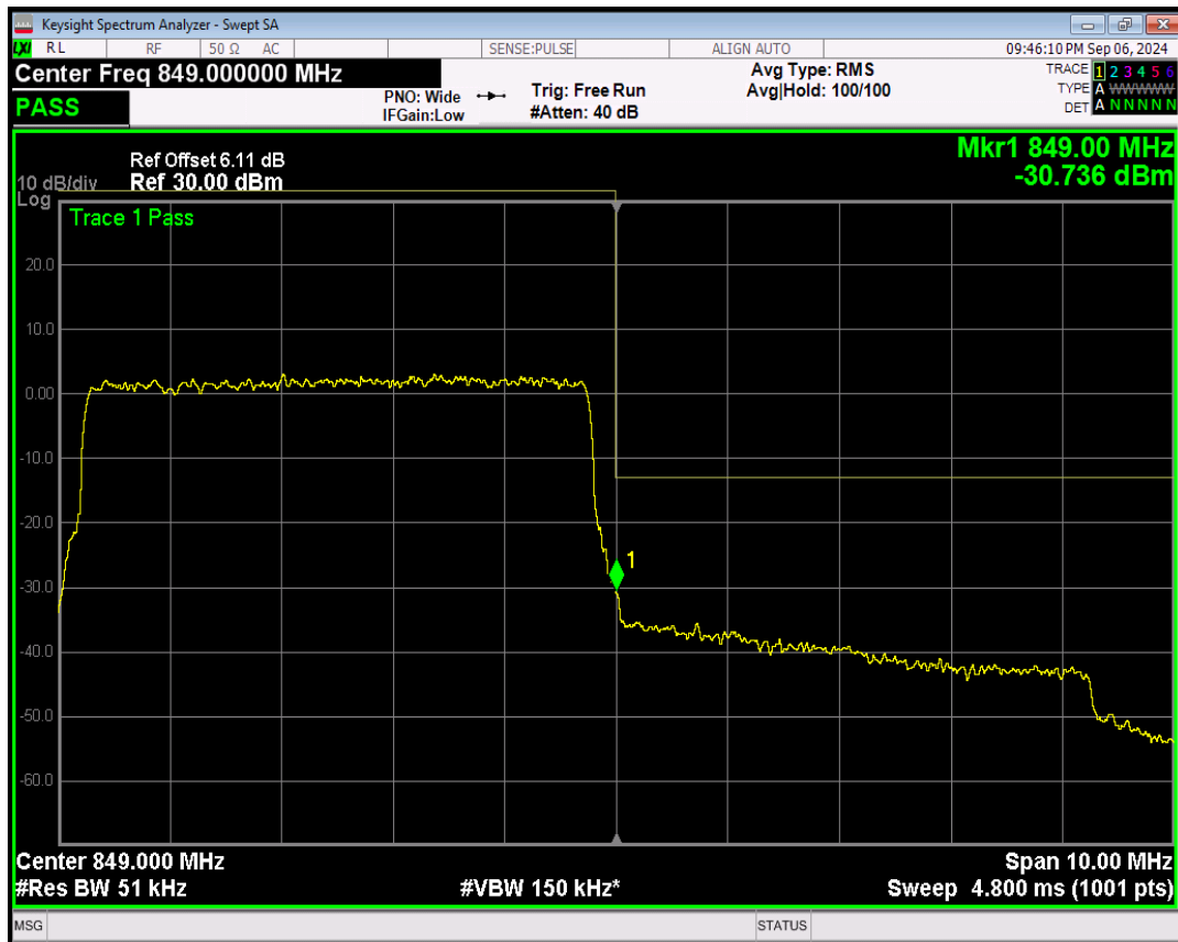
Band26(824-849) 16QAM BW=5MHz Channel=27015 RB Size=1 Position=#0
