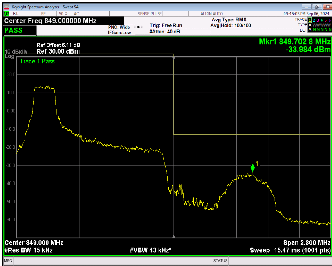
Band26(824-849) 16QAM BW=1.4MHz Channel=27033 RB Size=1 Position=#Max
