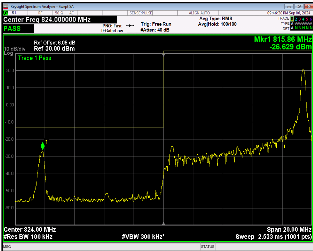
Band26(824-849) 16QAM BW=10MHz Channel=26840 RB Size=50 Position=#0
