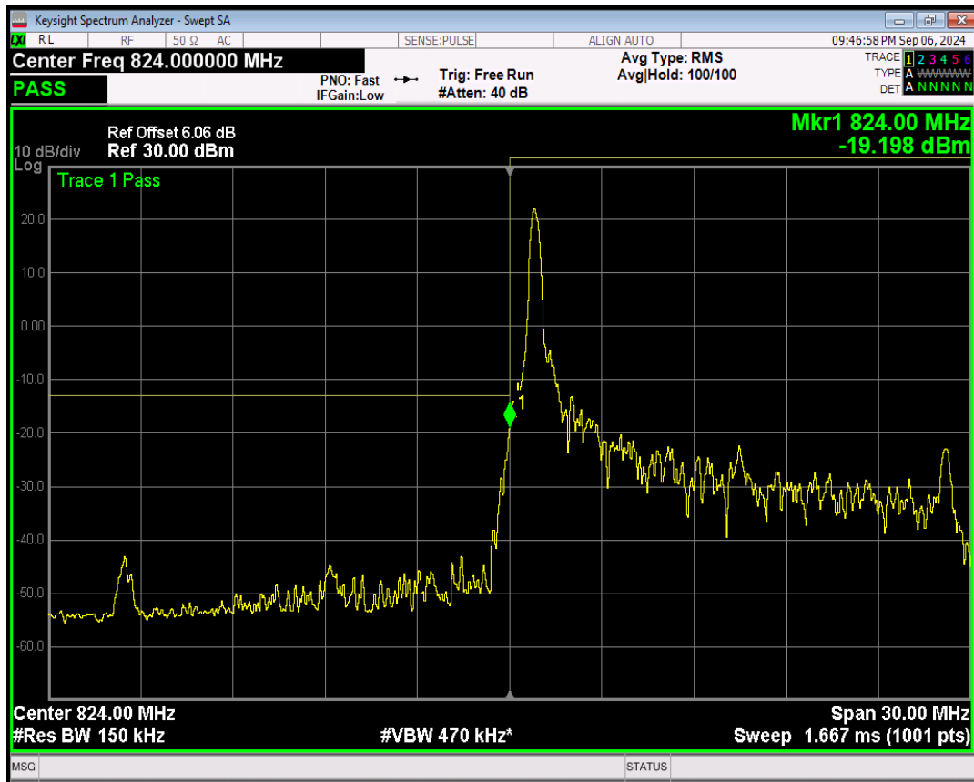
Band26(824-849) 16QAM BW=15MHz Channel=26865 RB Size=1 Position=#Max
