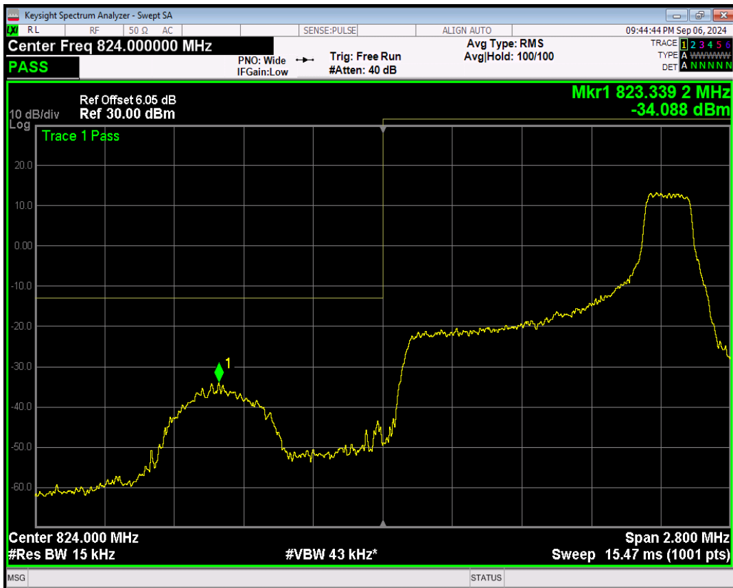
Band26(824-849) 16QAM BW=1.4MHz Channel=26797 RB Size=6 Position=#0
