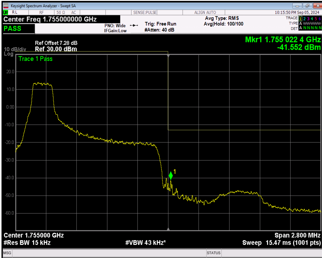
Band4 16QAM BW=1.4MHz Channel=20393 RB Size=1 Position=#Max
