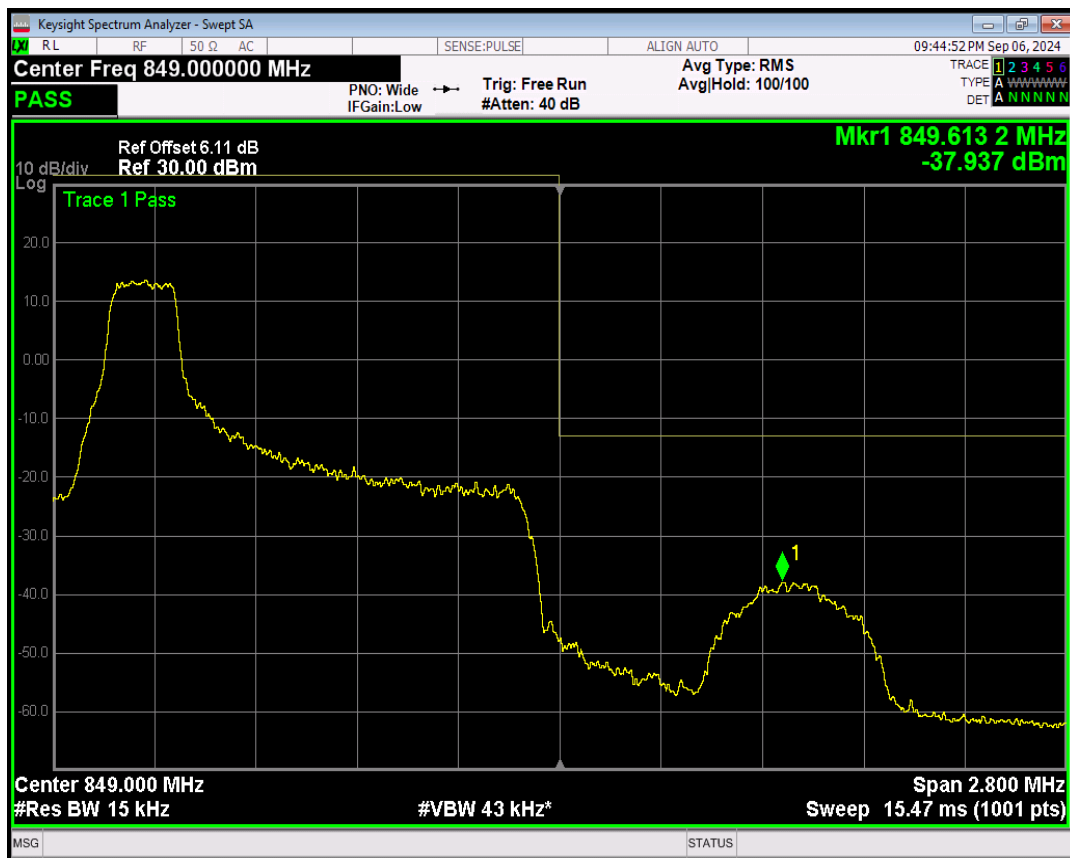
Band26(824-849) QPSK BW=1.4MHz Channel=27033 RB Size=1 Position=#Max
