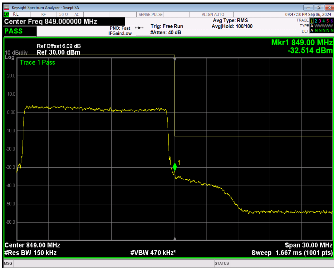
Band26(824-849) 16QAM BW=15MHz Channel=26965 RB Size=1 Position=#0
