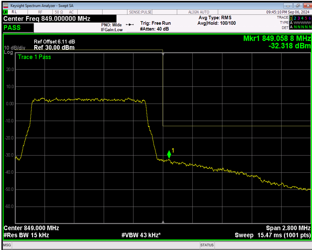
Band26(824-849) QPSK BW=3MHz Channel=26805 RB Size=1 Position=#0
