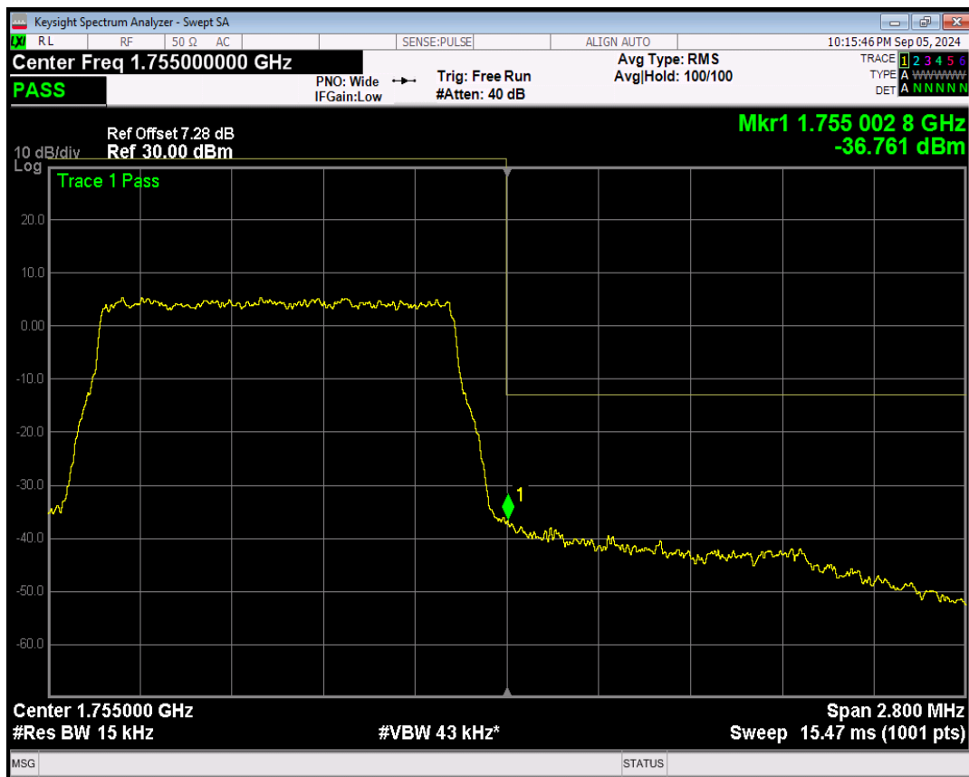
Band4 16QAM BW=1.4MHz Channel=20393 RB Size=1 Position=#0
