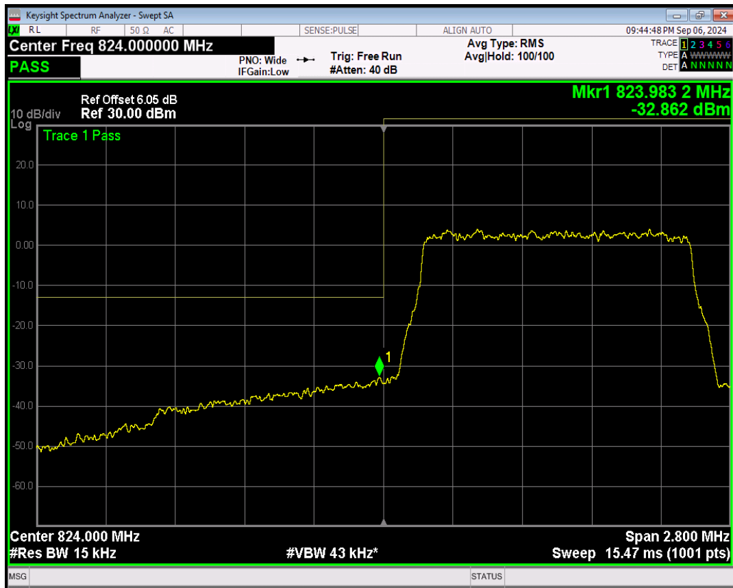
Band26(824-849) QPSK BW=1.4MHz Channel=27033 RB Size=1 Position=#0
