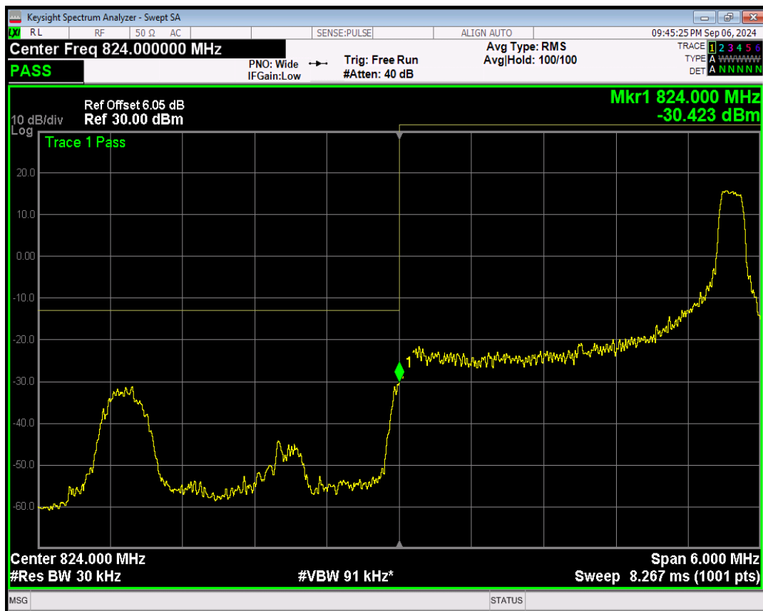
Band26(824-849) 16QAM BW=3MHz Channel=26805 RB Size=15 Position=#0
