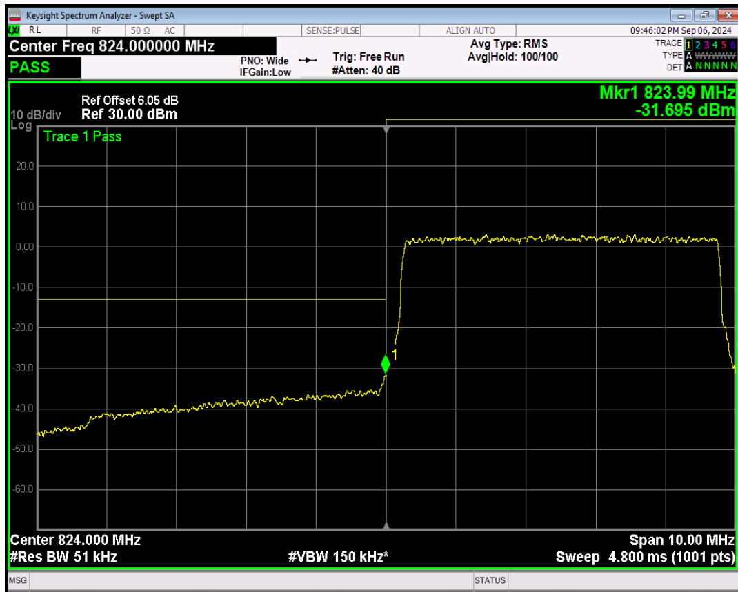
Band26(824-849) QPSK BW=5MHz Channel=27015 RB Size=1 Position=#0
