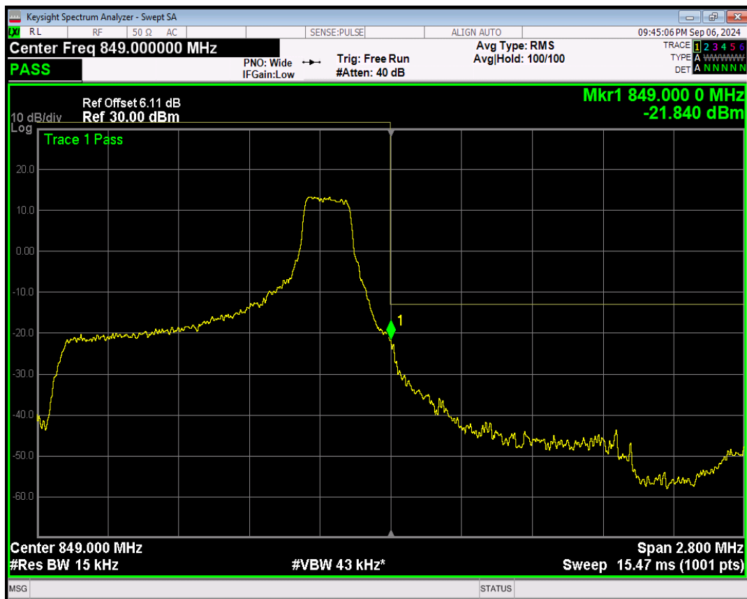
Band26(824-849) 16QAM BW=1.4MHz Channel=27033 RB Size=6 Position=#0
