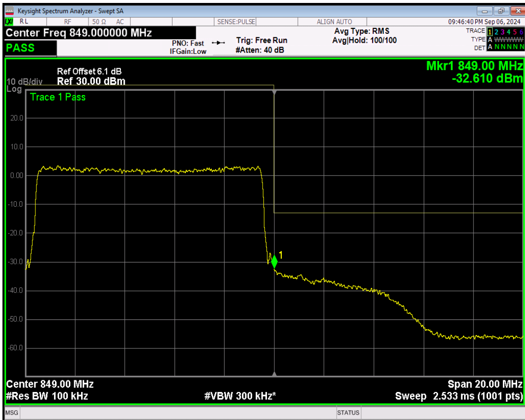
Band26(824-849) 16QAM BW=10MHz Channel=26990 RB Size=1 Position=#0
