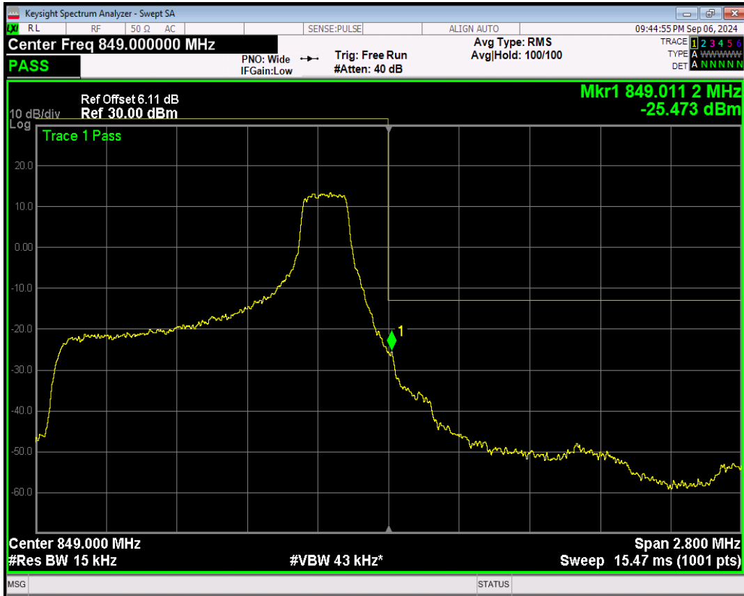
Band26(824-849) QPSK BW=1.4MHz Channel=27033 RB Size=6 Position=#0
