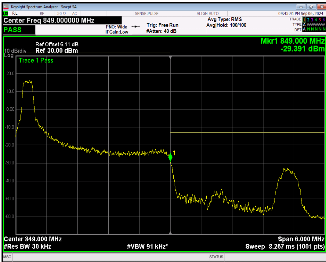
Band26(824-849) 16QAM BW=3MHz Channel=27025 RB Size=1 Position=#Max
