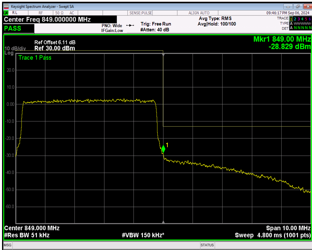
Band26(824-849) QPSK BW=10MHz Channel=26840 RB Size=1 Position=#0
