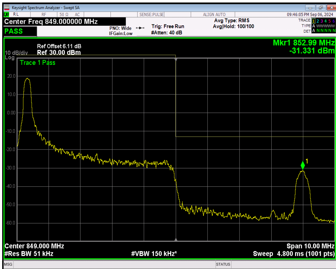
Band26(824-849) QPSK BW=5MHz Channel=27015 RB Size=1 Position=#Max
