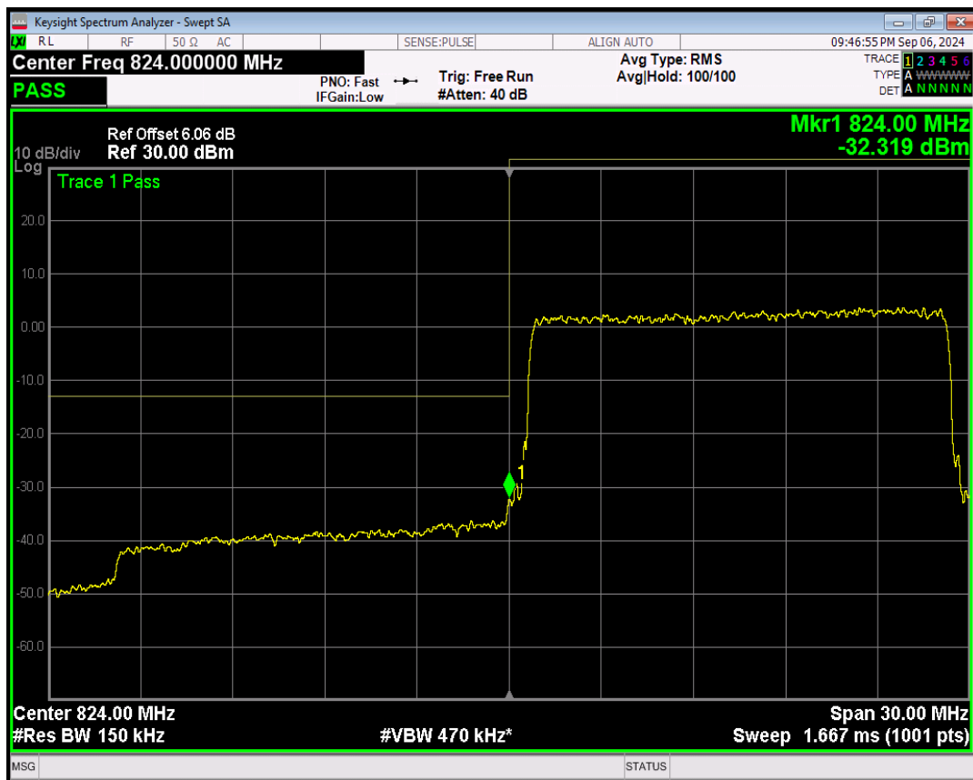
Band26(824-849) 16QAM BW=15MHz Channel=26865 RB Size=1 Position=#0
