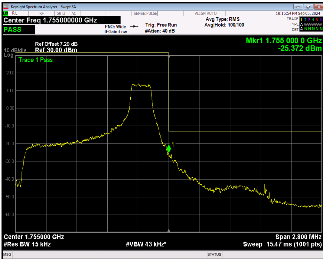
Band4 16QAM BW=1.4MHz Channel=20393 RB Size=6 Position=#0
