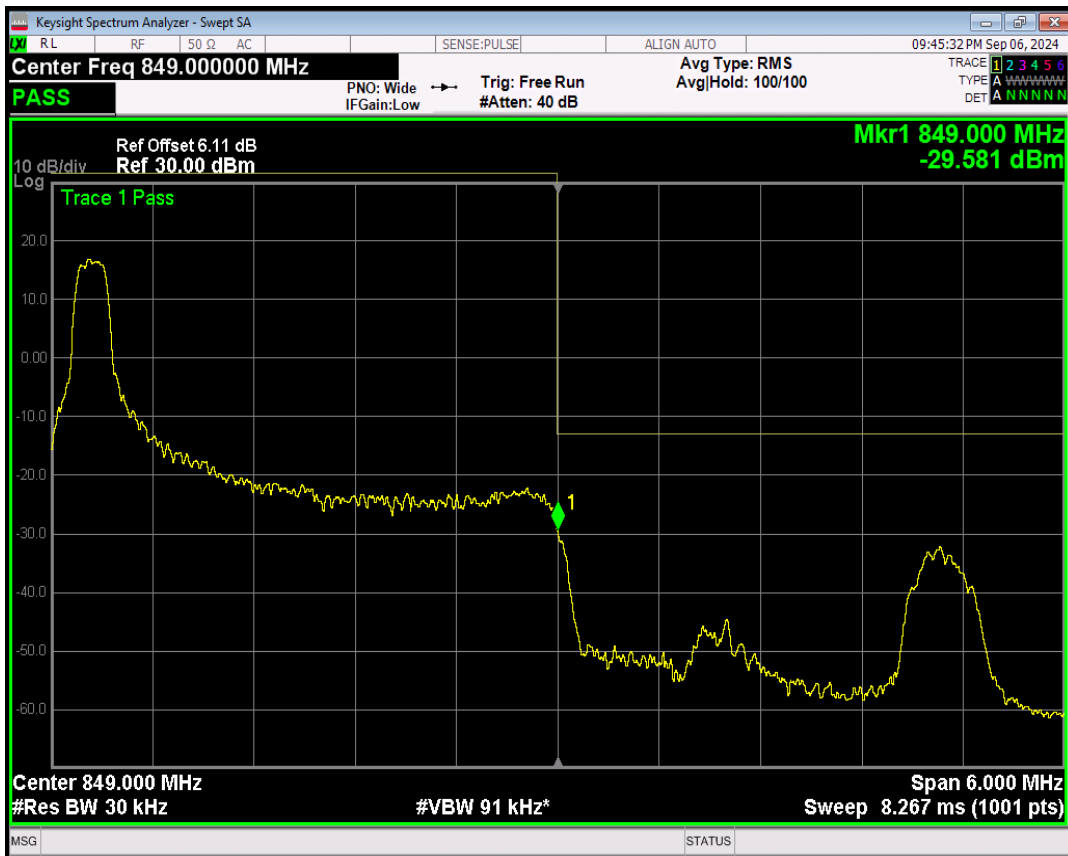
Band26(824-849) QPSK BW=3MHz Channel=27025 RB Size=1 Position=#Max
