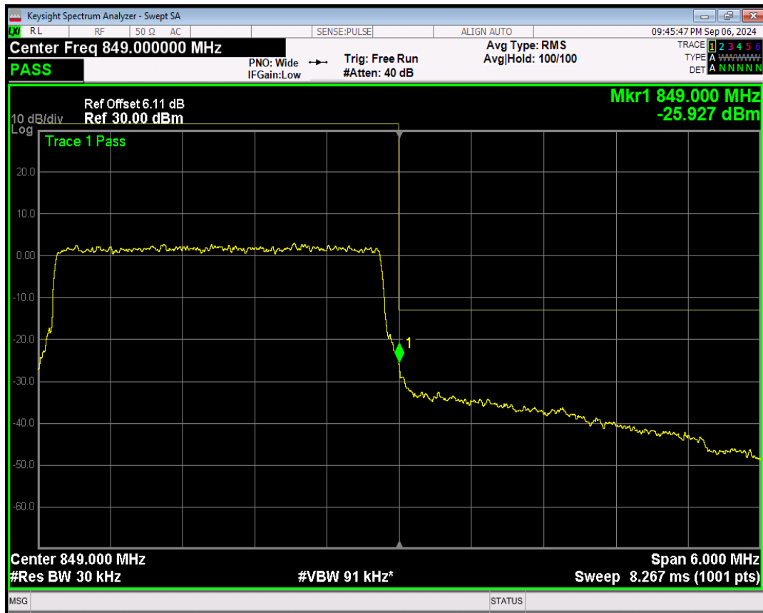
Band26(824-849) QPSK BW=5MHz Channel=26815 RB Size=1 Position=#0
