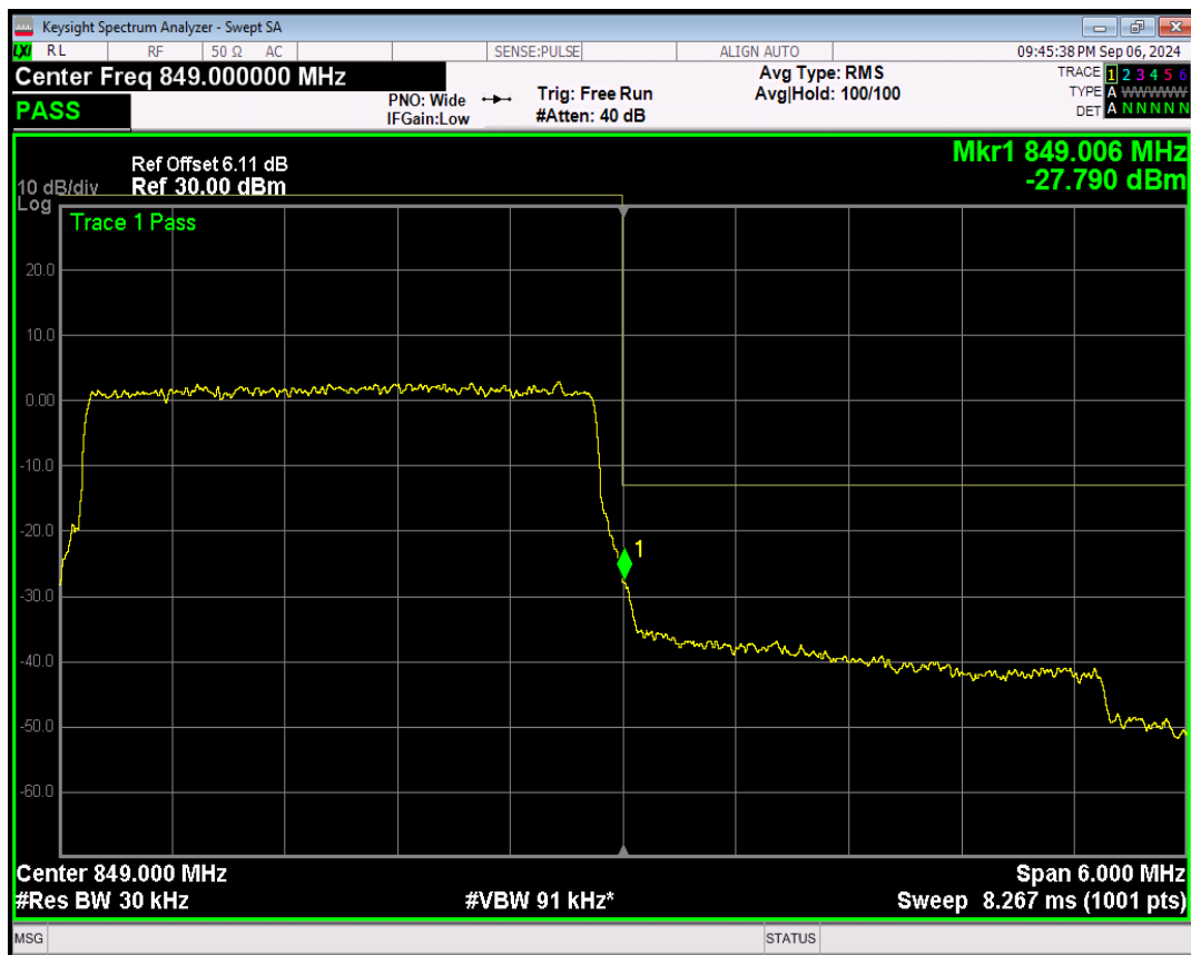
Band26(824-849) 16QAM BW=3MHz Channel=27025 RB Size=1 Position=#0
