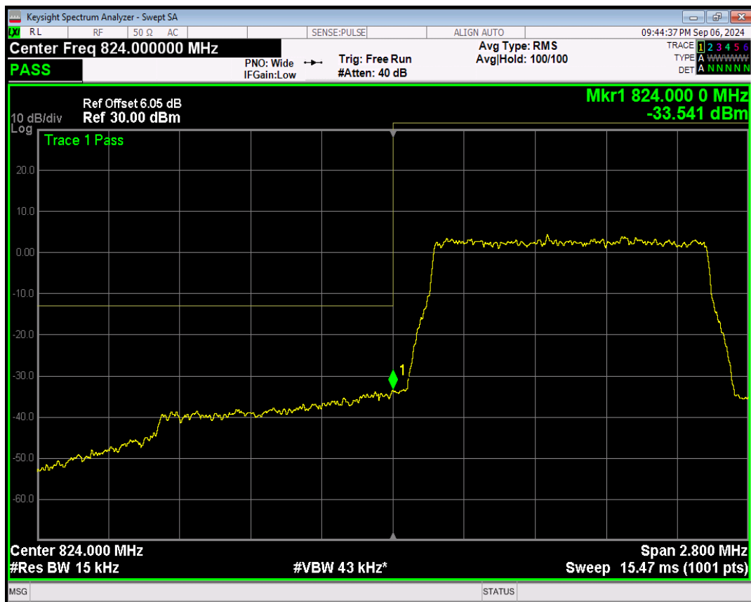
Band26(824-849) 16QAM BW=1.4MHz Channel=26797 RB Size=1 Position=#0
