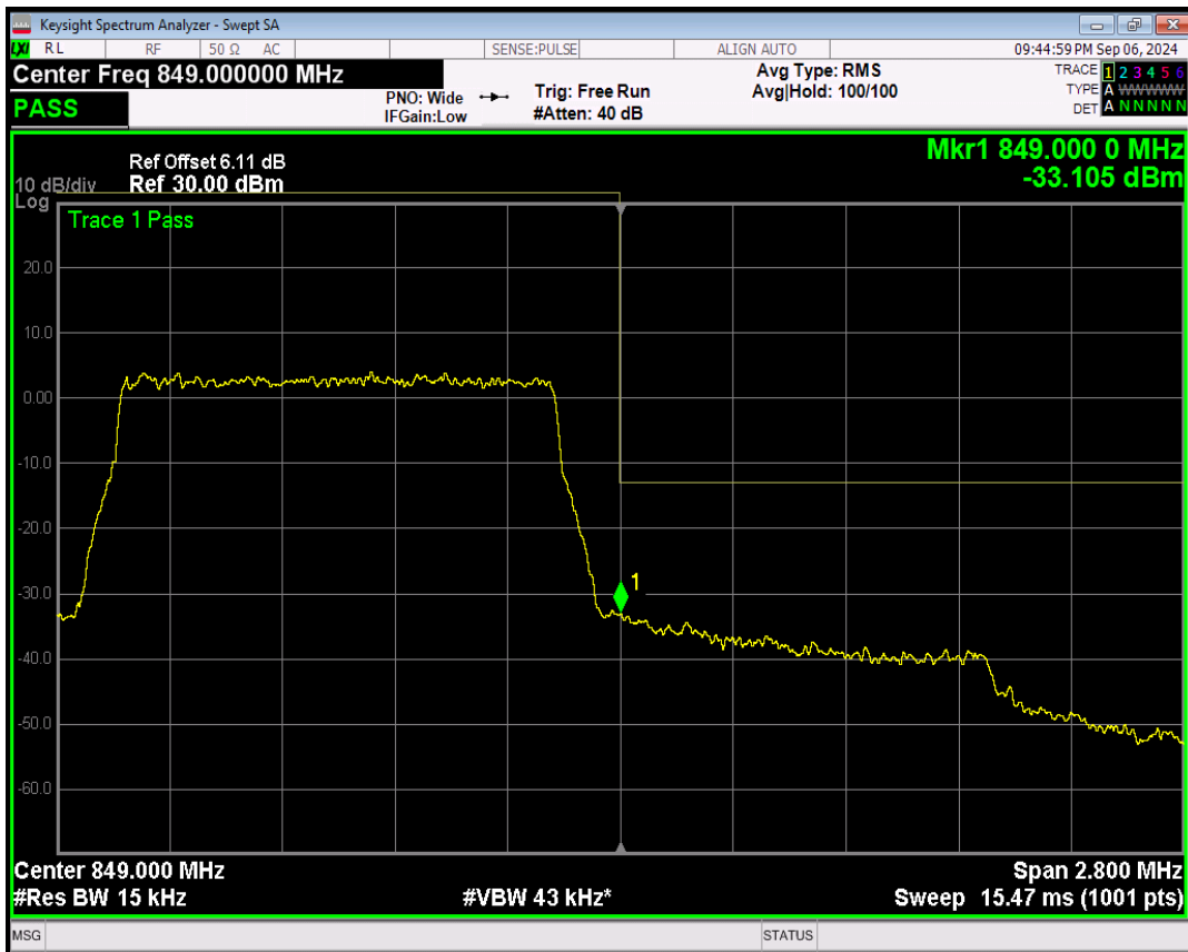
Band26(824-849) 16QAM BW=1.4MHz Channel=27033 RB Size=1 Position=#0
