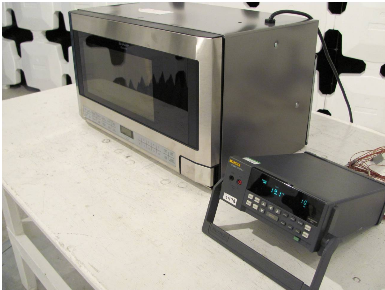
Figure 7. Output Power Test Configuration
