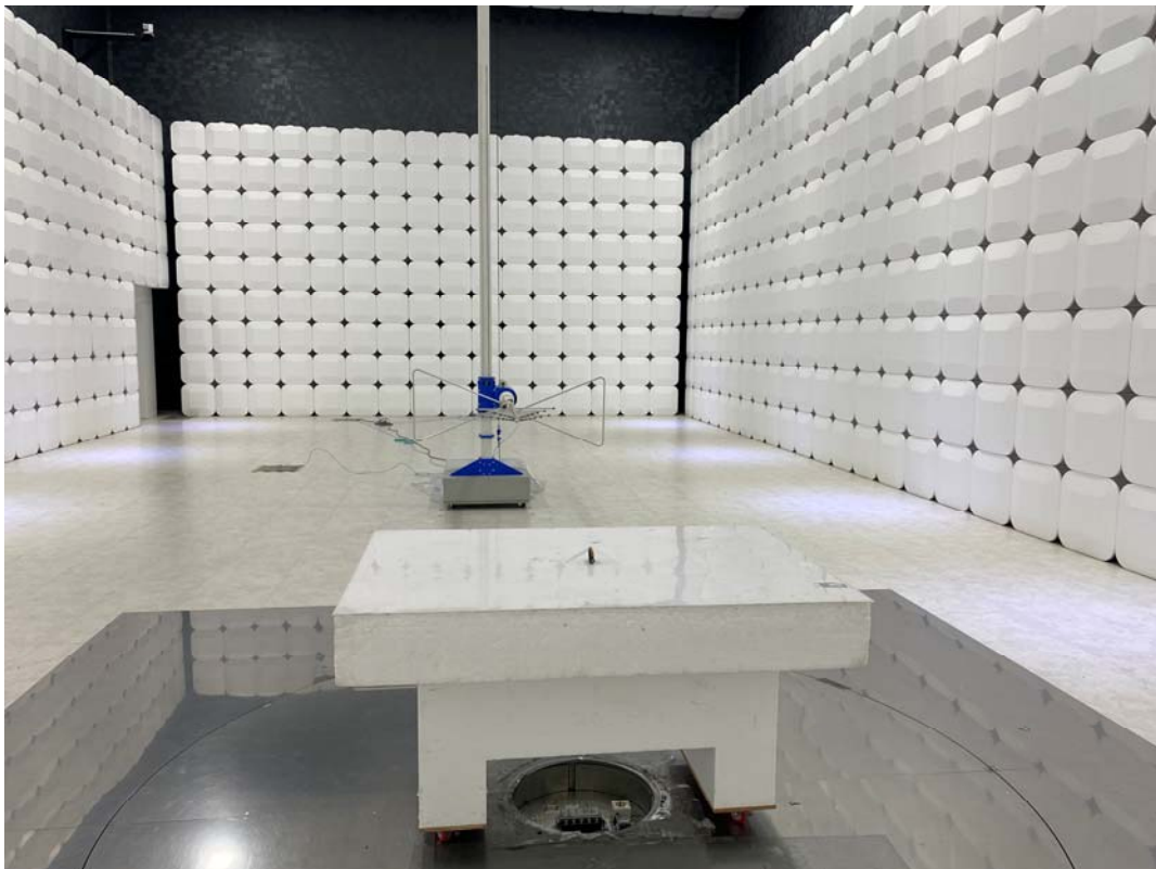
Radiated emission test (30 MHz to 1 GHz)
