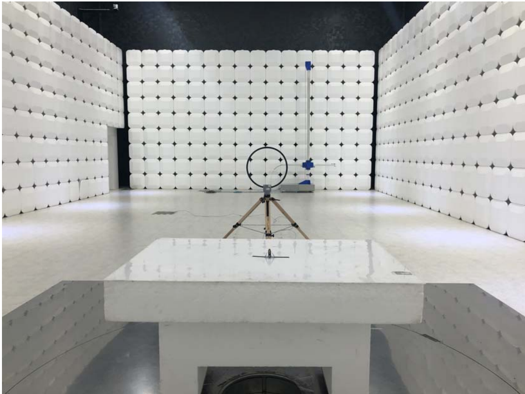
Radiated emission test (9 kHz to 30 MHz)
