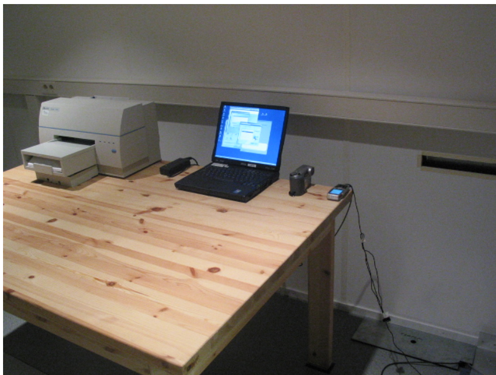
Picture 3 AC powerline conducted emission measurement (BlueTooth)
