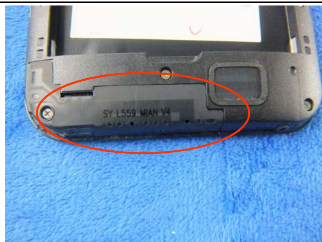
GSM/PCS/UMTS-FDD Antenna View
