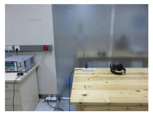
FCC RADIATED EMISSION TEST SETUP
