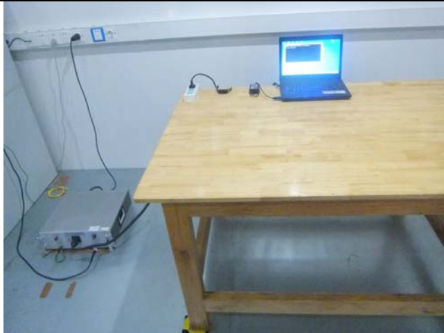
Conducted Emissions Test Setup Front View
