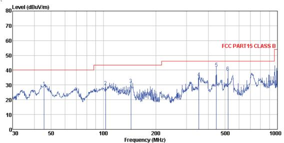
: 3m chamber : FCC PART15 CLASS B 3m VULB9163-2013M VERTICAL : Burnning test mode :: Rong Site Condition Test mode Test Engin
