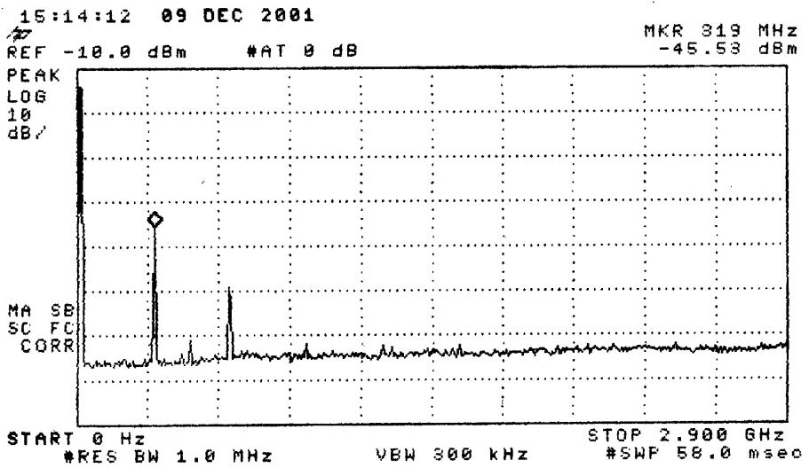
Figure 6.2(b). Emission spectrum of the DUT (310 MHz, 50% duty factor).
