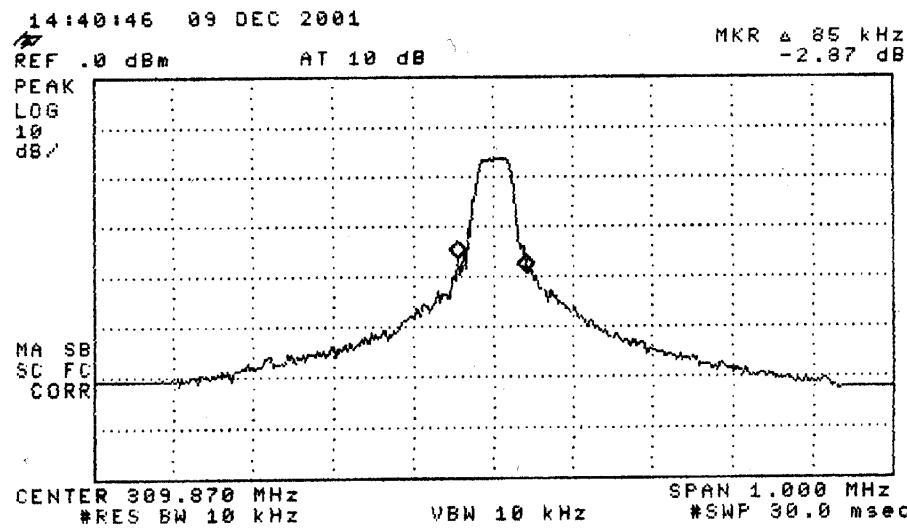
Figure 6.3(a). Measured bandwidth of the DUT.
