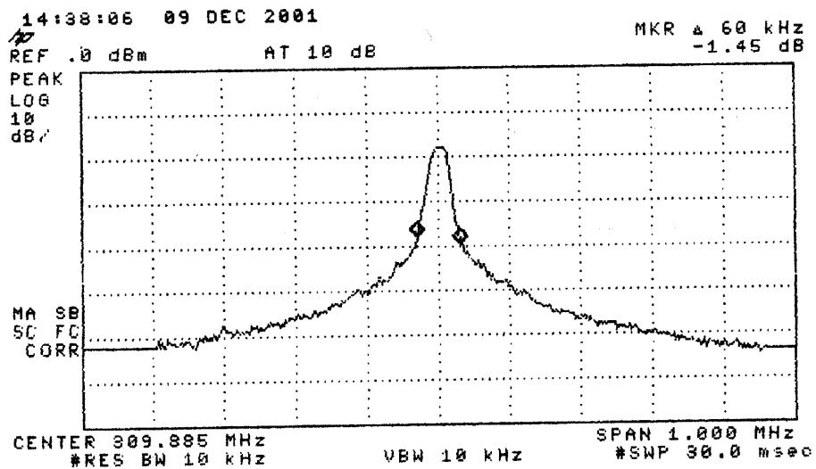
Figure 6.3(c). Measured bandwidth of the DUT.
