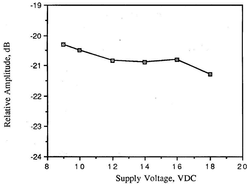
Figure 6.4. Relative emission vs. supply voltage. (310 MHz, continuous pulsed)
