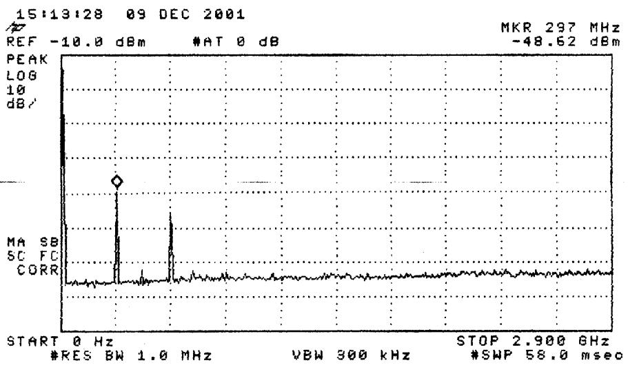
Figure 6.2(a). Emission spectrum of the DUT (288 MHz, 50% duty factor).
