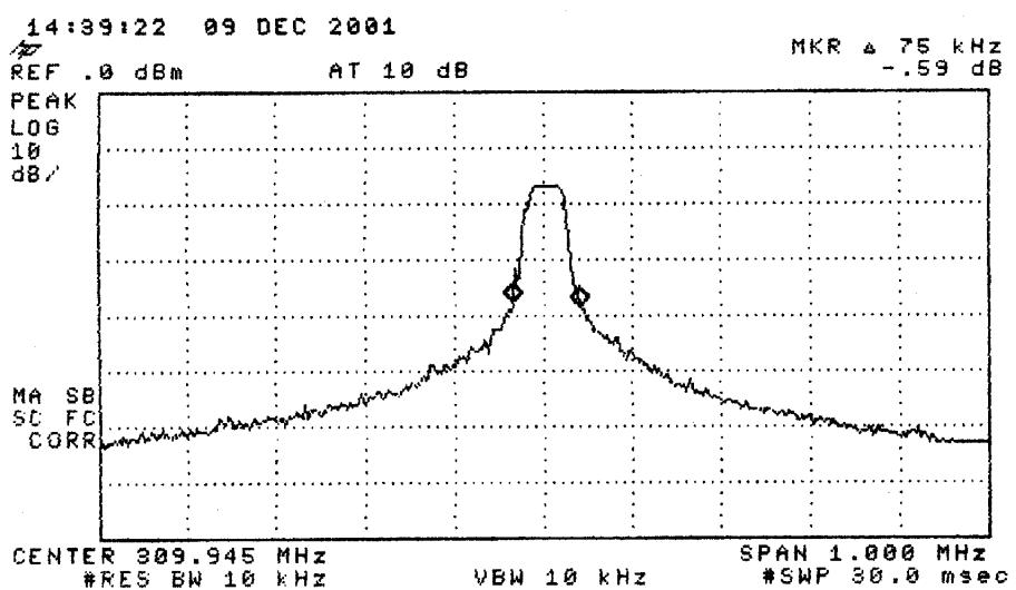
Figure 6.3(b). Measured bandwidth of the DUT.
