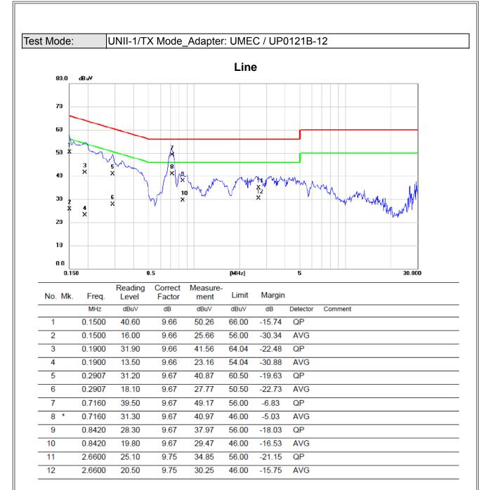
Note: The test result has included the cable loss.
