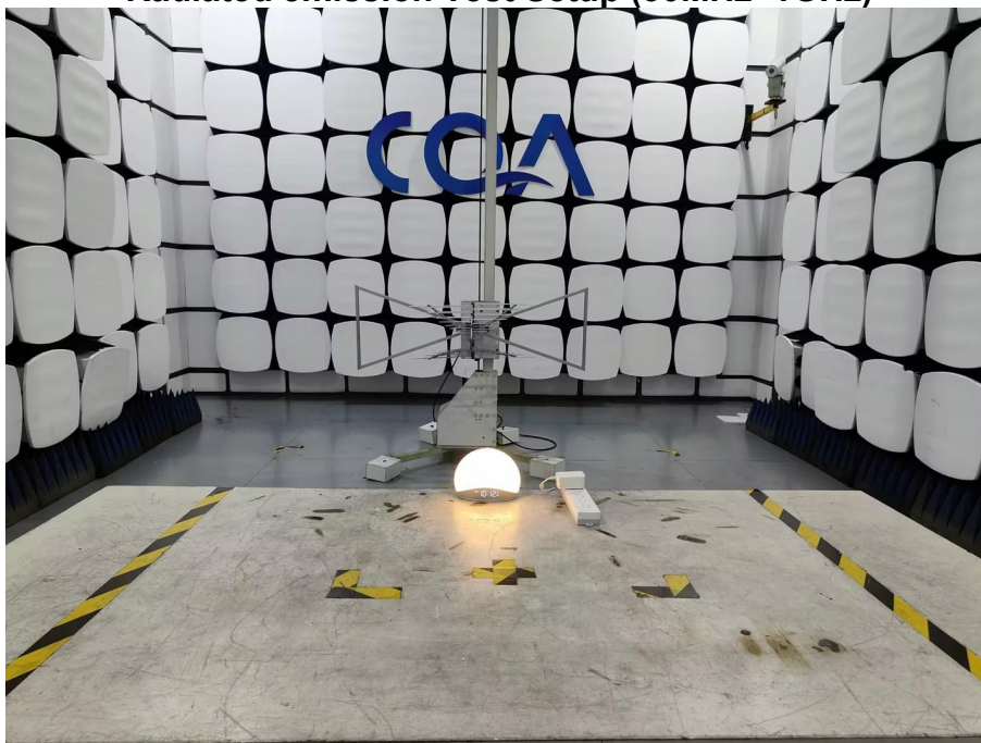
Radiated emission Test Setup (30MHz~1GHz)
