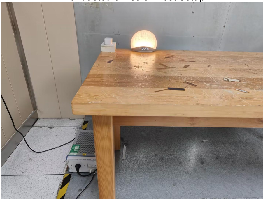
Conducted emission Test Setup
