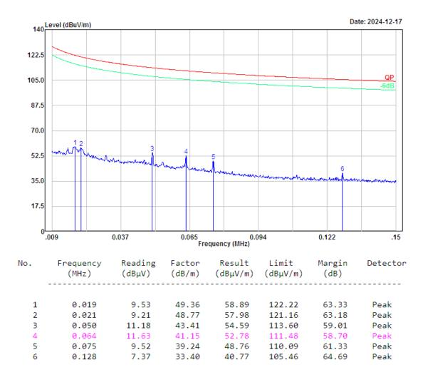
Project No.: 2402A107821E-RF Polarization: Parallel Test Mode: Transmitting : RBW:10kHz VBW:30kHz Serial No.: 2VBI-3 Tester: Alan Xie
