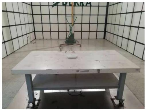
Description: Radiated Emission Test Setup for 1~18GHz(AP410C)
