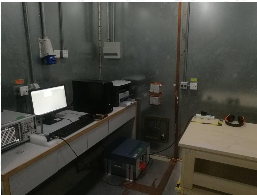
FCC RADIATED EMISSION TEST SETUP
