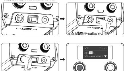
CCT mode setting: Press MODE button to CCT mode, rotate "Right knob" to select from DIM, CCT and G/M, rotate "Left knob" to adjust the value of DIM, CCT and G/M. DIM range: 000%...100%, CCT range: 01800K...20000K, G/M range: -100...+100
