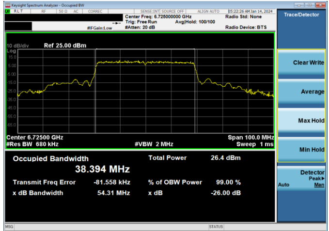
Plot 7-40. 26dB & 99% Bandwidth Plot Antenna WF5B (40MHz 802.11ax RU484 (UNII Band 7) - Ch. 155)
