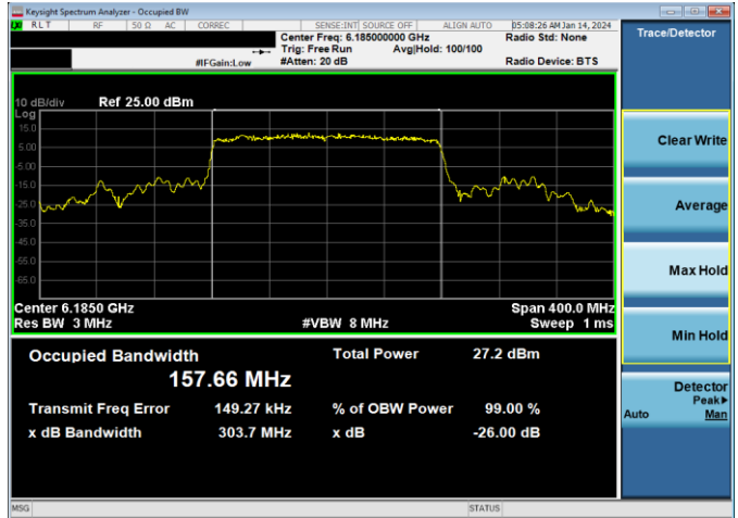
Plot 7-16. 26dB & 99% Bandwidth Plot Antenna WF5B (160MHz 802.11ax RU996x2 (UNII Band 5) – Ch. 47)
