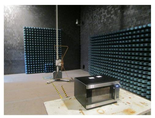
2. Radiated Emission Measurement above 1GHz
