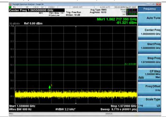
Simultaneous / Spurious / 700 MHz + 800 MHz / Downlink / 1 Carrier / Additional 1559 MHz ~ 1572 MHz
