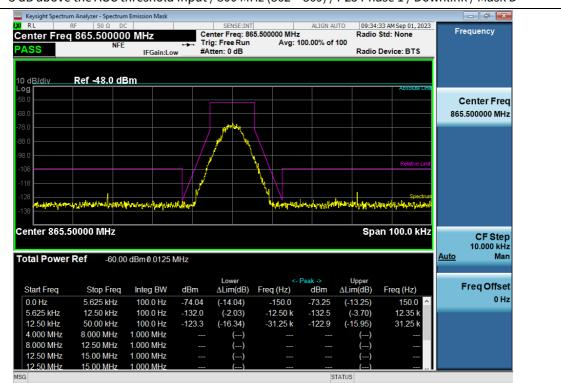
3 dB above the AGC threshold Input / 800 MHz (862 ~ 869) / P25 Phase 1 / Downlink / Mask D
