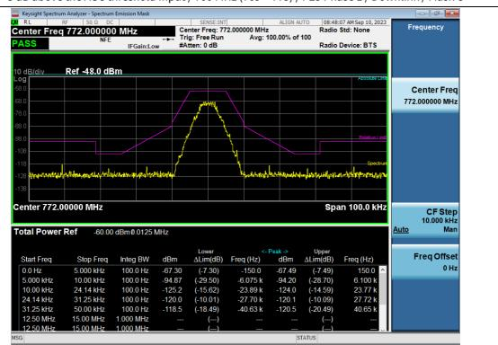
3 dB above the AGC threshold Input / 700 MHz (769 ~ 775) / P25 Phase 1 / Downlink / Mask C
