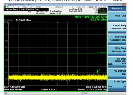
Spurious / 700 MHz (799 ~ 805) / Uplink / 1 Carrier / Additional 1585 MHz ~ 1598 MHz
