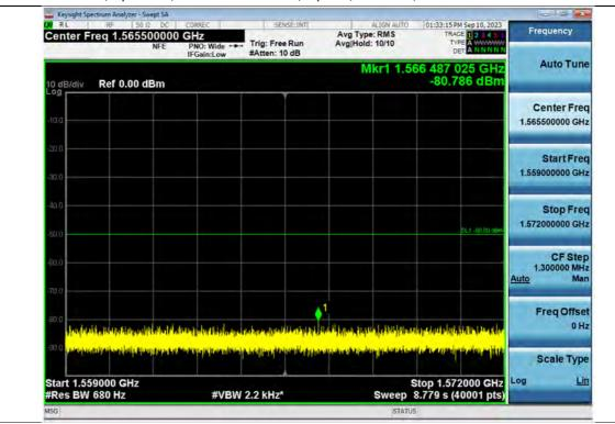
Simultaneous / Spurious / 700 MHz + 800 MHz / Uplink / 1 Carrier / Additional 1559 MHz ~ 1572 MHz
