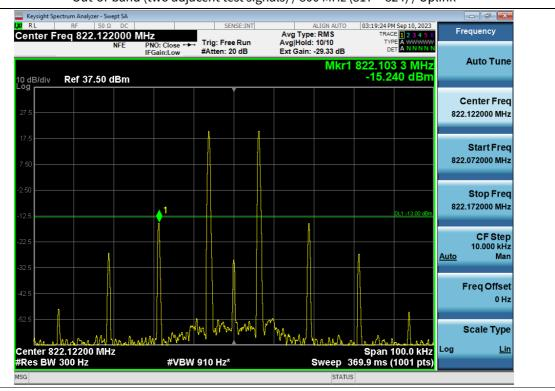
Out-of-band (two adjacent test signals) / 800 MHz (817 ~ 824) / Uplink
