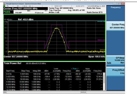
3 dB above the AGC threshold Input / 800 MHz (854 ~ 861) / P25 Phase 1 / Downlink / Mask D
