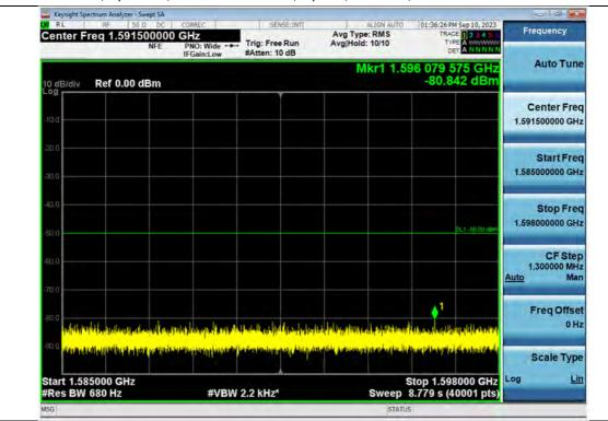
Simultaneous / Spurious / 700 MHz + 800 MHz / Uplink / 1 Carrier / Additional 1585 MHz ~ 1598 MHz
