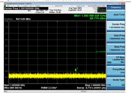
Spurious / 700 MHz (769 ~ 775) / Downlink / 1 Carrier / Additional 1585 MHz ~ 1598 MHz
