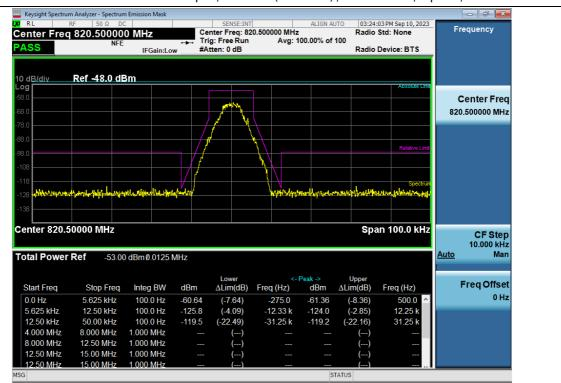
3 dB above the AGC threshold Input / 800 MHz (817 ~ 824) / P25 Phase 1 / Uplink / Mask D
