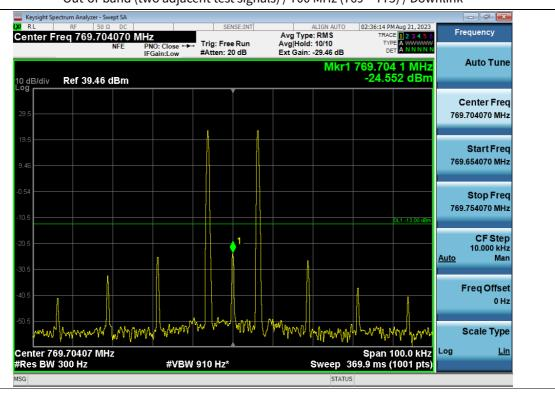
Out-of-band (two adjacent test signals) / 700 MHz (769 ~ 775) / Downlink
