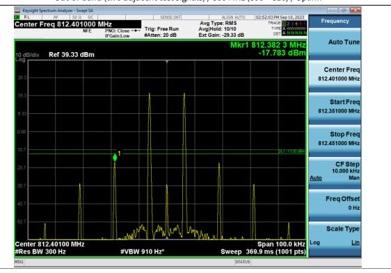
Out-of-band (two adjacent test signals) / 800 MHz (806 ~ 816) / Uplink
