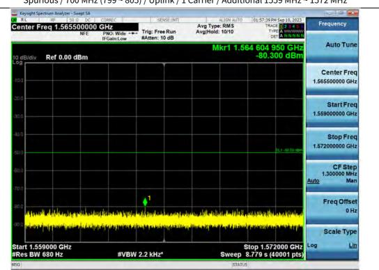
Spurious / 700 MHz (799 ~ 805) / Uplink / 1 Carrier / Additional 1559 MHz ~ 1572 MHz
