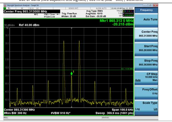
Out-of-band (two adjacent test signals) / 800 MHz (862 ~ 869) / Downlink
