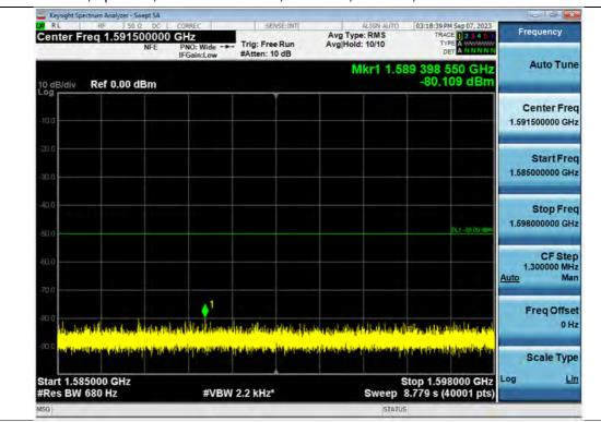
Simultaneous / Spurious / 700 MHz + 800 MHz / Downlink / 1 Carrier / Additional 1585 MHz ~ 1598 MHz
