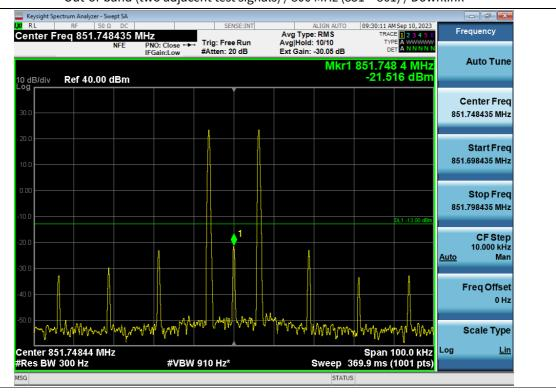
Out-of-band (two adjacent test signals) / 800 MHz (851 ~ 861) / Downlink
