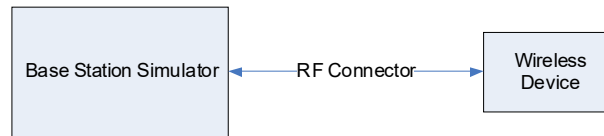
Figure 9-3 Power Measurement Setup
