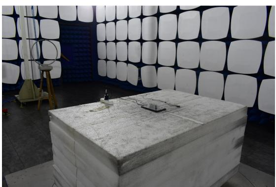
3. Radiated emission (9KHz-30MHz)
