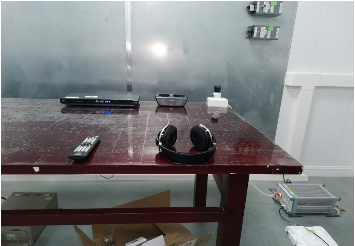
Photograph 3: Set-up photo for Conducted Emission on AC Mains
