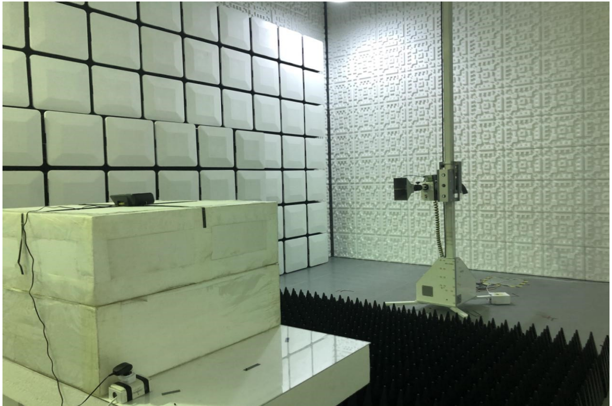
Photograph 2: Set-up photo for Radiated Spurious Emission, above 1GHz
