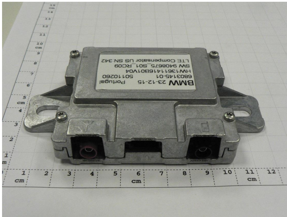
Photograph: 3: connectors side – RF and power supply
