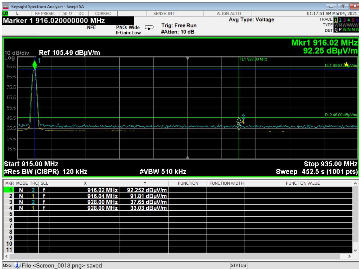
Band Edge – 916 MHz – Vertical Polarization – Y-Axis
