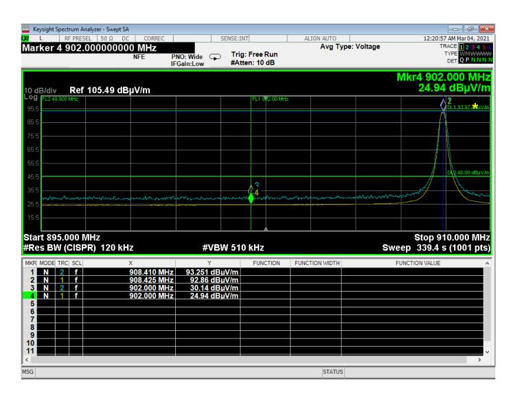
Band Edge – 908.42 MHz – Vertical Polarization – Y-Axis
