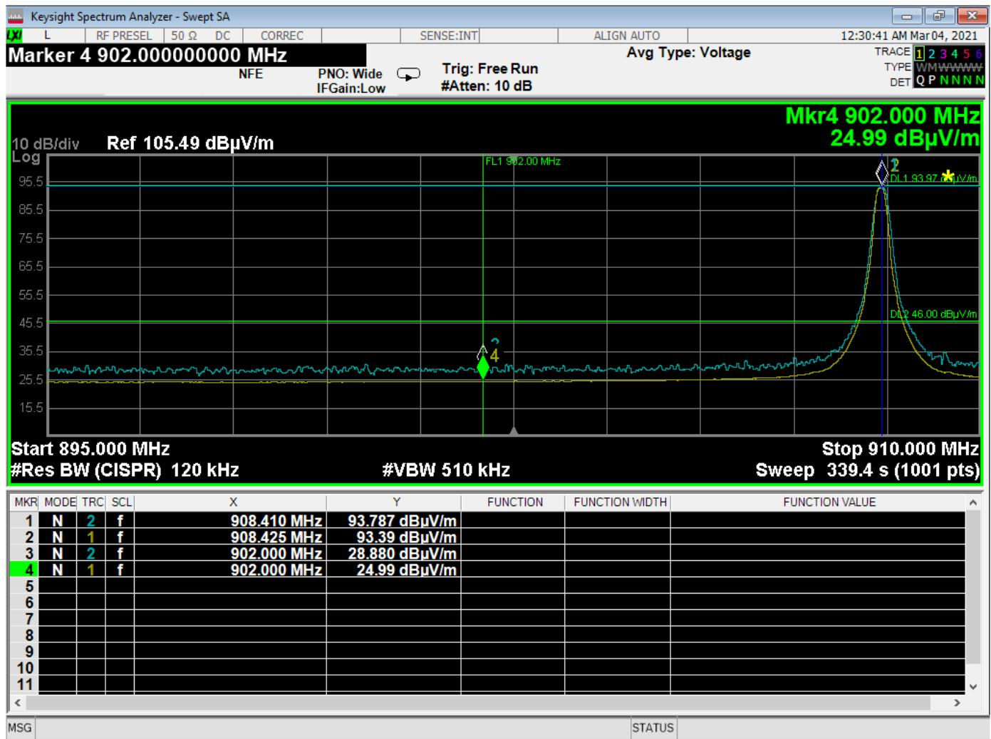
Band Edge – 908.42 MHz – Horizontal Polarization – X-Axis
