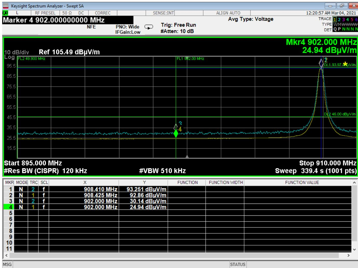
Band Edge – 908.42 MHz – Vertical Polarization – Y-Axis
