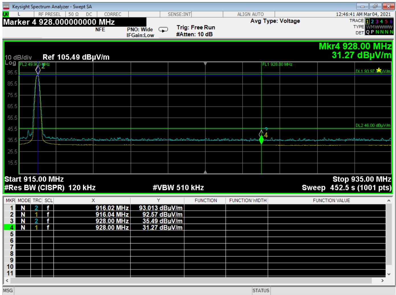
Band Edge – 916 MHz – Horizontal Polarization – X-Axis
