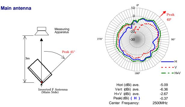
Note1) The measurement was performed at 3 frequencies (2400, 2450, 2500MHz). Note2) The maximum antenna gain was found around **45 degree** angle from measuring apparatus in **horizontal** polarization at the middle frequency (2500MHz).
