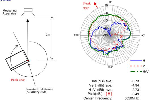
Note1) The measurement was performed at 4 frequencies (5725, 5750, 5800, 5850MHz). Note2) The maximum antenna gain was found around **335 degree** angle from measuring apparatus in **vertical** polarization at the middle frequency (5850MHz).
