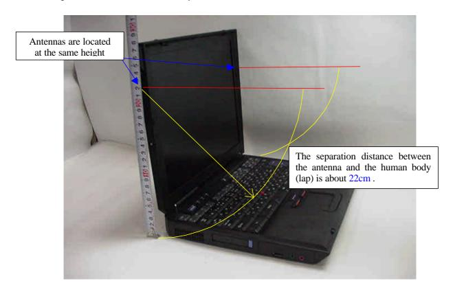
The highest conducted peak output power of the Test Report is 53.7mW (17.3dBm) and the maximum antenna gain is 0.85 dBi (See page 4 of this exhibit.).
