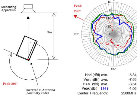
Note1) The measurement was performed at 3 frequencies (2400, 2450, 2500MHz). Note2) The maximum antenna gain was found around **295 degree** angle from measuring apparatus in **horizontal** polarization at the middle frequency (2500MHz).
