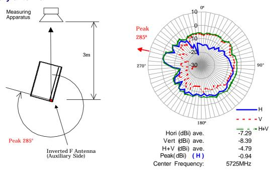
Note1) The measurement was performed at 4 frequencies (5725, 5750, 5800, 5850MHz). Note2) The maximum antenna gain was found around **285 degree** angle from measuring apparatus in **horizontal** polarization at the middle frequency (5725MHz).
