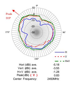
Note1) The measurement was performed at 3 frequencies (2400, 2450, 2500MHz). Note2) The maximum antenna gain was found around **315 degree** angle from measuring apparatus in **vertical** polarization at the middle frequency (2450MHz).
