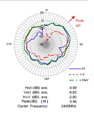
Note1) The measurement was performed at 3 frequencies (2400, 2450, 2500MHz). Note2) The maximum antenna gain was found around **45 degree** angle from measuring apparatus in **horizontal** polarization at the middle frequency (2400MHz).
