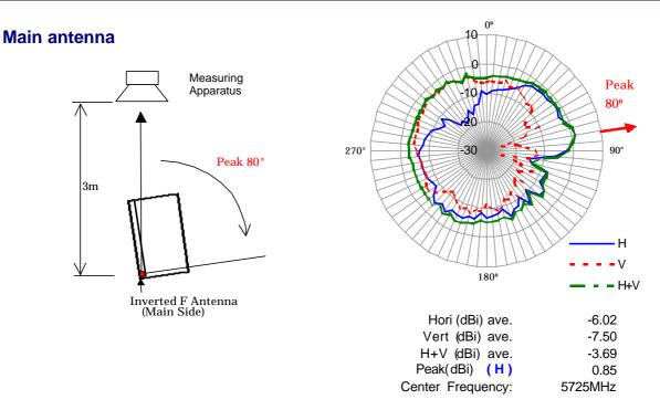
Note1) The measurement was performed at 4 frequencies (5725, 5750, 5800, 5850MHz). Note2) The maximum antenna gain was found around **80 degree** angle from measuring apparatus in **horizontal** polarization at the middle frequency (5725MHz).
