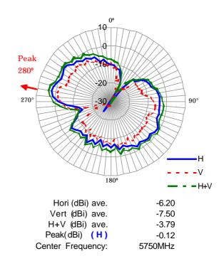
Note1) The measurement was performed at 4 frequencies (5725, 5750, 5800, 5850MHz). Note2) The maximum antenna gain was found around **280 degree** angle from measuring apparatus in **horizontal** polarization at the middle frequency (5750MHz).
