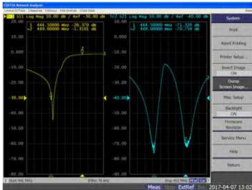
Figure 27: Rejection of Each Port for UHF Duplexer
