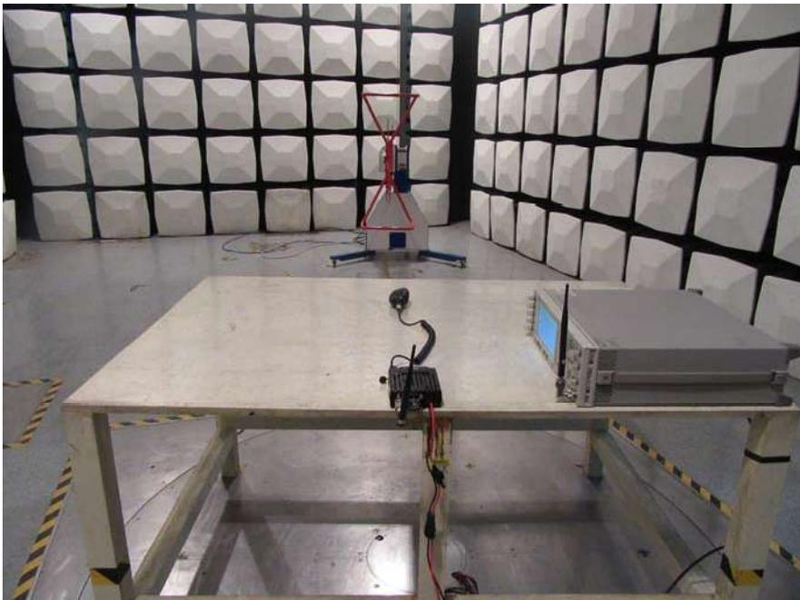
**Radiated Emission - Front View (Above 1 GHz)**
