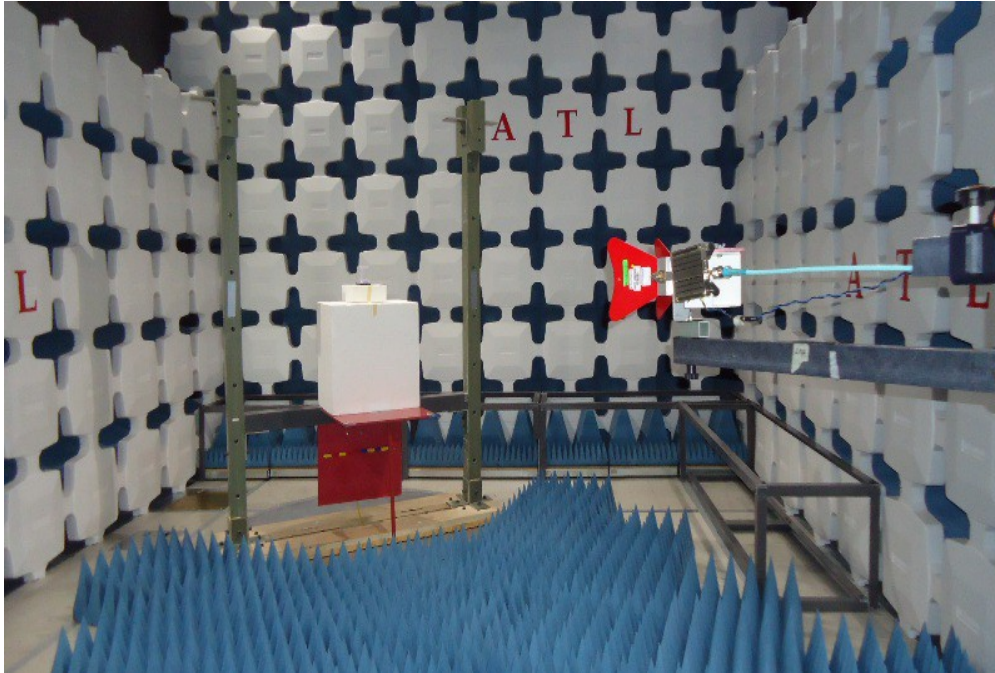
Figure 4.4 - Radiated Emission Test Setup - Front View
