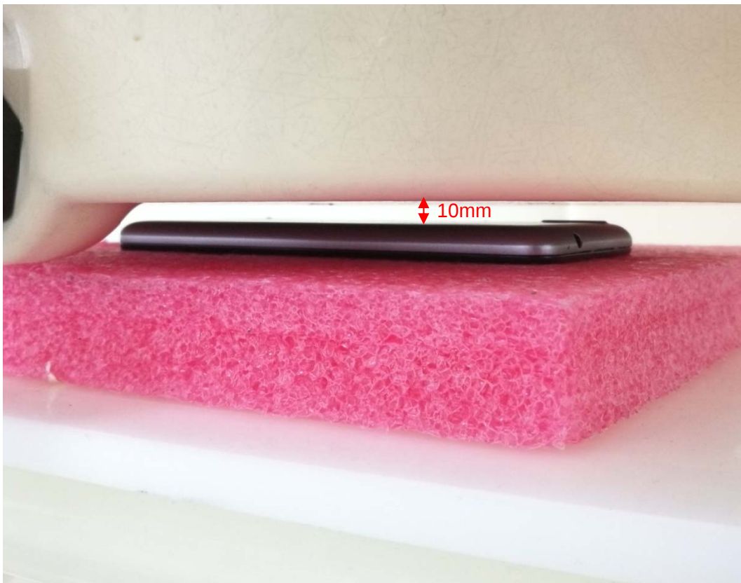
Picture 6: Back Side without holder, the distance from handset to the bottom of the Phantom is 10mm
