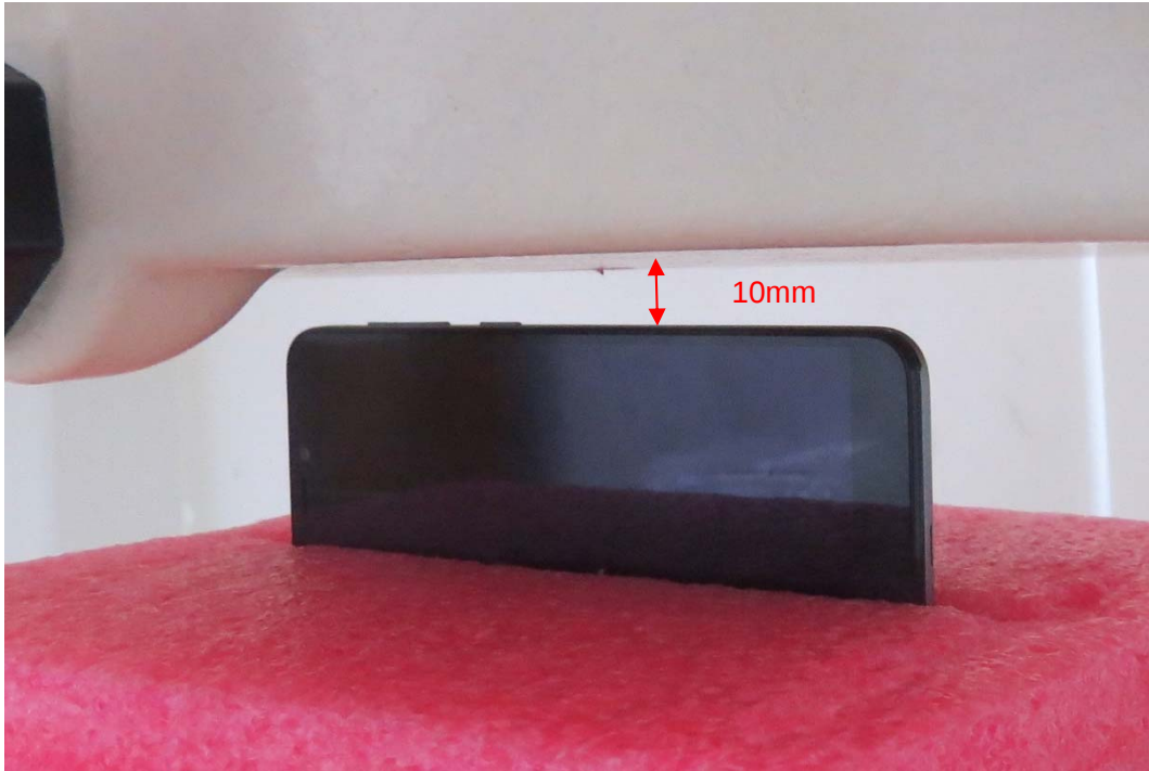
Picture 9: Right Side, the distance from handset to the bottom of the Phantom is 10mm
