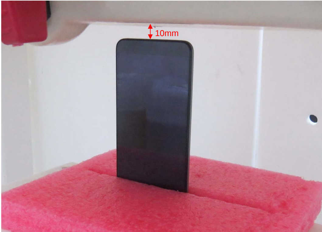
Picture 11: Bottom Edge, the distance from handset to the bottom of the Phantom is 10mm
