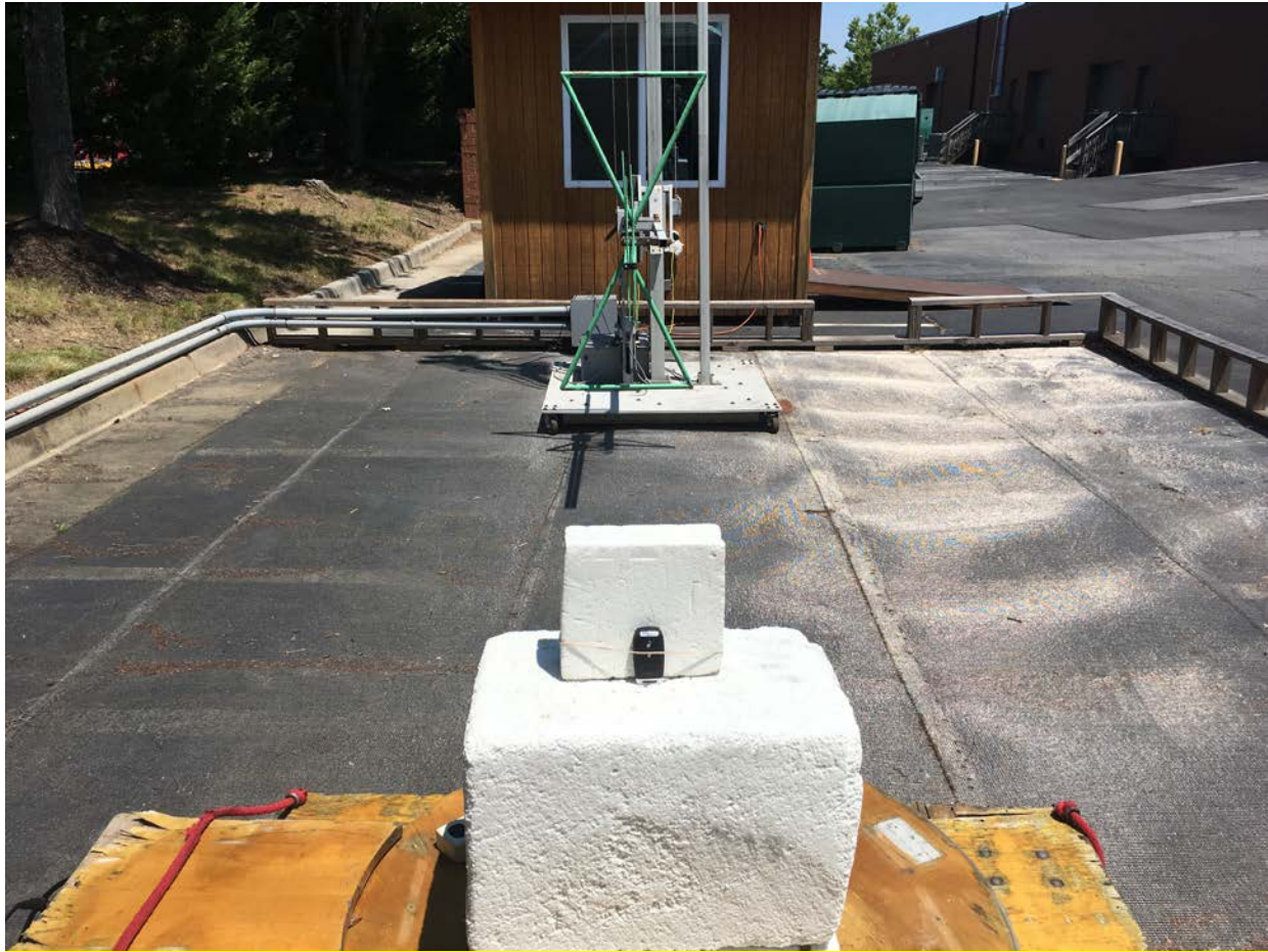
Photograph 1: Radiated Testing – Front View (Less than 1 GHz)
