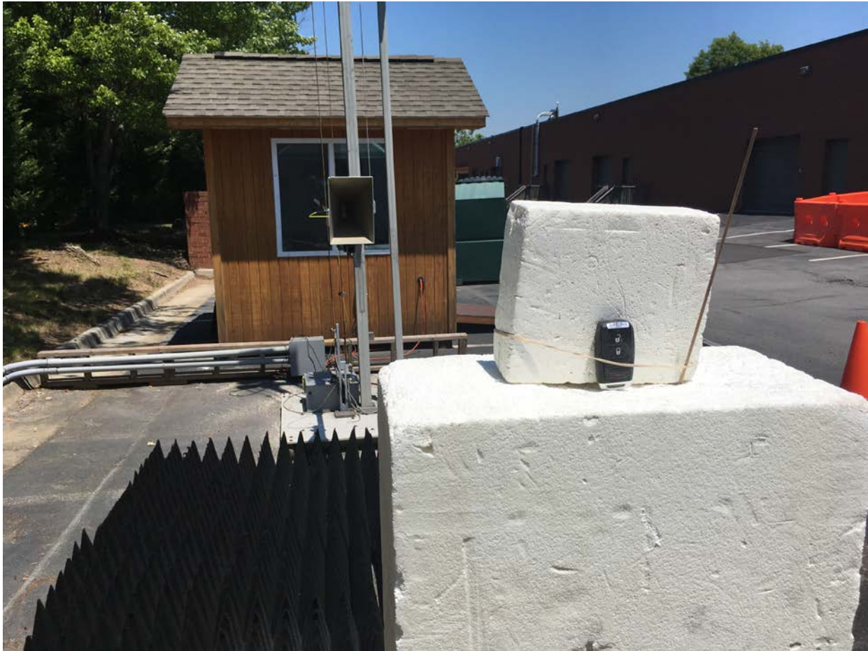
Photograph 2: Radiated Testing – Front View (Greater than 1 GHz)
