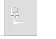
Peel off the protective layer from the double sided tape on the back of the SwitchBot Lock stand, align the back of the stand to the alignment card's square and stick it onto your door.
