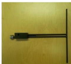
**Figure 1** – MVG COMOSAR Validation Dipole
