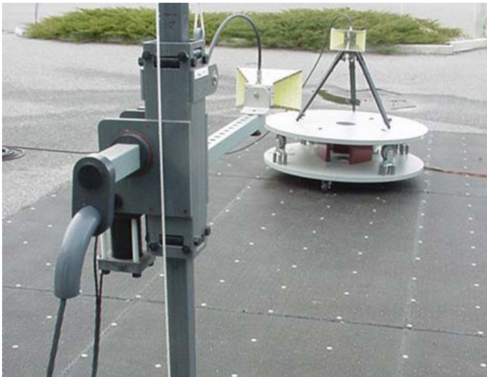
Signal Substitution Test Setup Photograph - Horn Antenna
