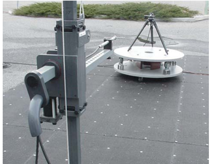
Signal Substitution Test Setup Photograph - Dipole Antenna
