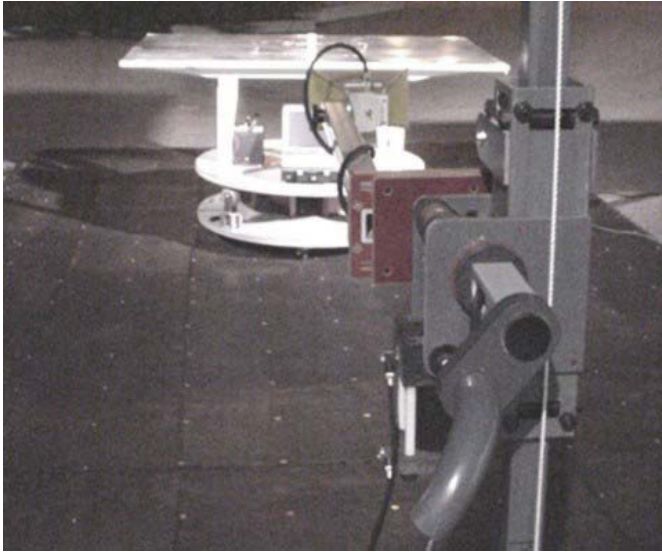
Radiated Measurement Test Setup Photograph - Horn Antenna
