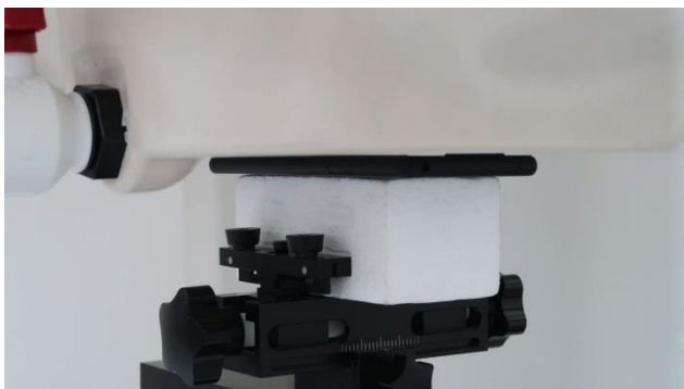
Back, Test Separation 0 mm
