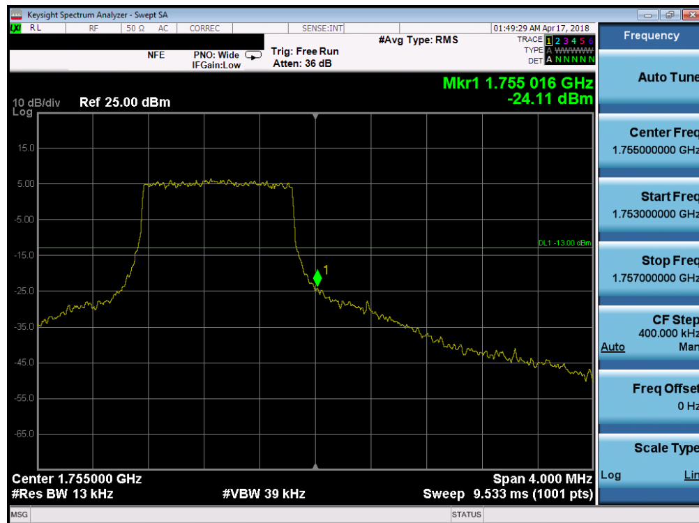
Plot 7-97. Upper Band Edge Plot (Band 4 - 1.4MHz QPSK - Full RB Configuration)
