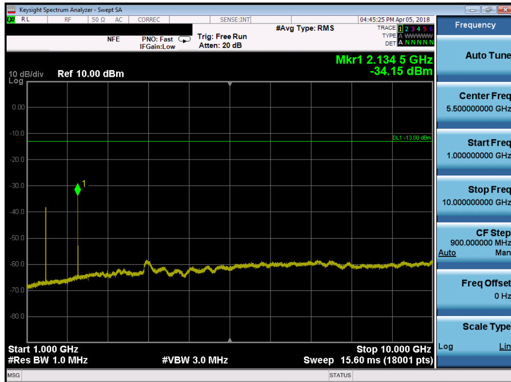
Plot 7-49. Conducted Spurious Plot (Band 12 - 5.0MHz QPSK - RB Size 1, RB Offset 0 - High Channel)
