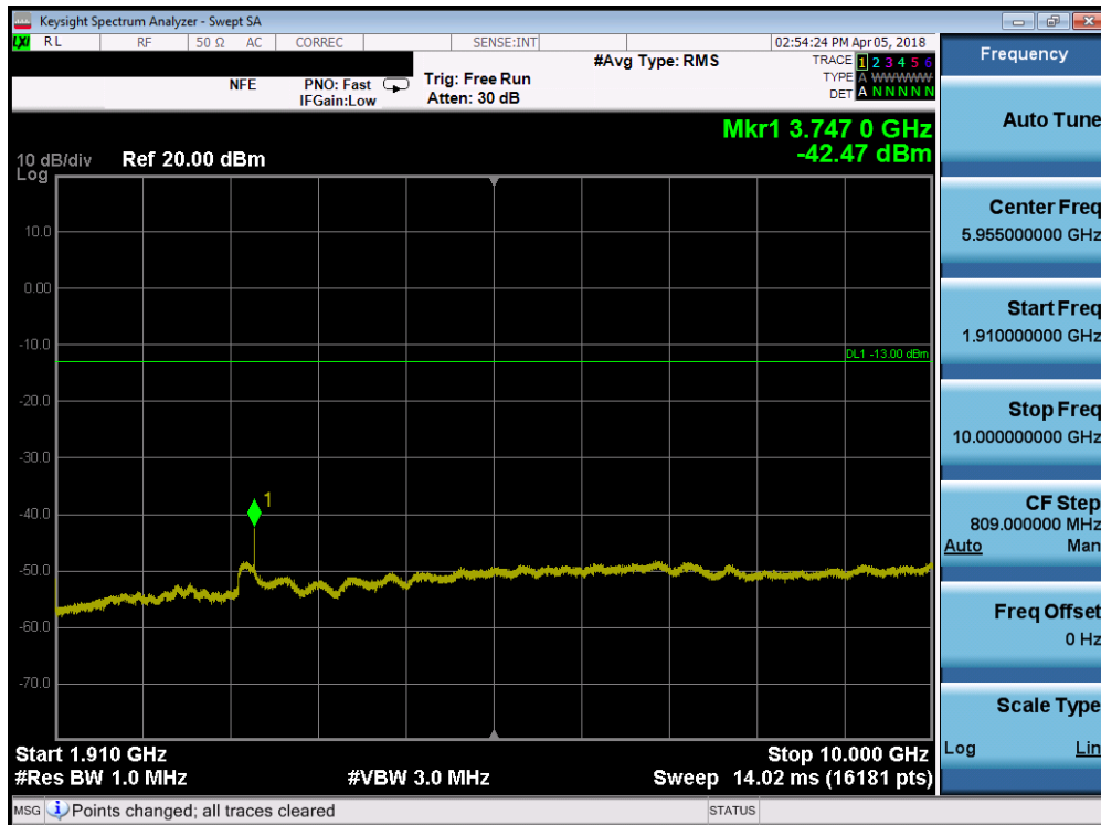
Plot 7-72. Conducted Spurious Plot (Band 2 - 15.0MHz QPSK - RB Size 1, RB Offset 0 - Mid Channel)
